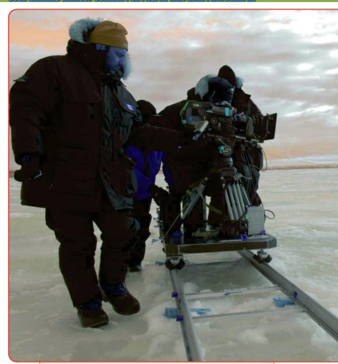
One job of the key grip is to build tracks and dollies for moving camera shots. These pieces of equipment allow cameras to move smoothly and easily during filming.
