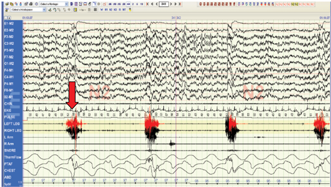
Figure 11.2 Sequence of four periodic limb movements of sleep from a polysomnography recording (gray arrow illustrates the first limb movement). (See insert for color representation of the figure.)
