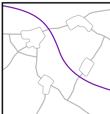
Figure 6.21-b Tangential route running between settlements.
