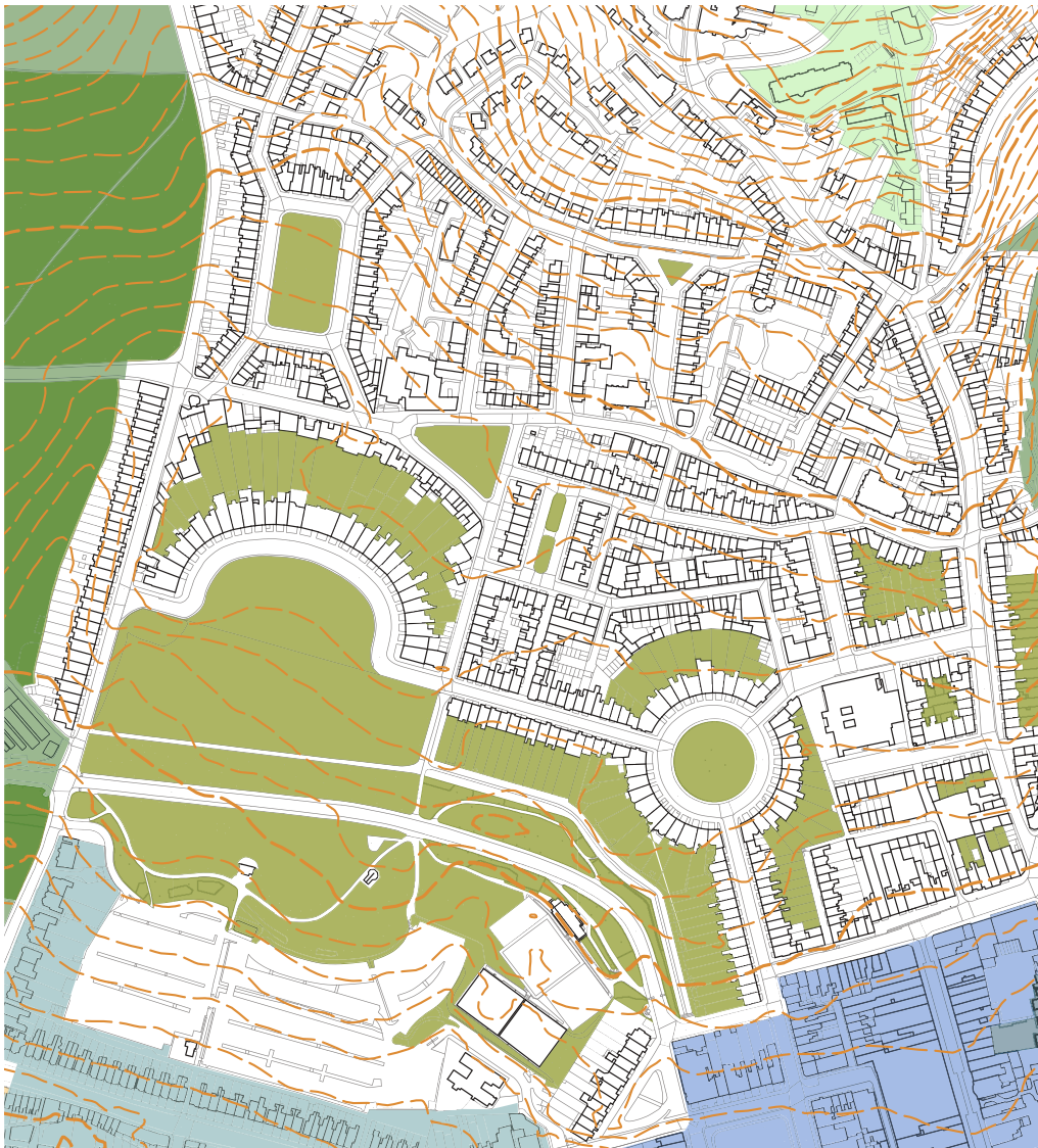
Figure 8.14-g Composite plan with overlays of contour lines and green spaces. Despite forming clear geometric shapes, the street pattern is inflected to adapt to the topography with streets running predominantly at right angles or parallel to the contours. The public green spaces are shaped and enclosed by the buildings and plots.
