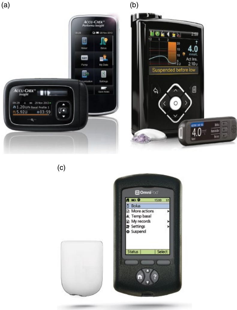
Figure 8.1 Some insulin pumps. (a) Pump with remote control device (AccuChek Insight [Roche]); (b) sensor-augmented pump (MiniMed 640G ® ) with SmartGuard ® – software that pauses insulin delivery if hypoglycaemia is predicted low (low-glucose suspend); (c) Patch pump (mylife OmniPod [Ypsomed]).
