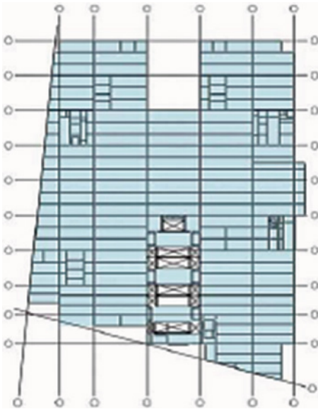
(b) Typical superstructure floors: large open floor plates, though moderated spans to balance loading between new raft and existing buttress foundations.
