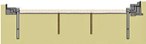
(d) Secant pile trim, capping beam, and temporary propping installation (supported on temporary piles at centre).
