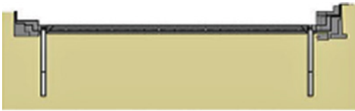
(c) Second stage demolition/clearance to central area of existing reinforced concrete raft.
