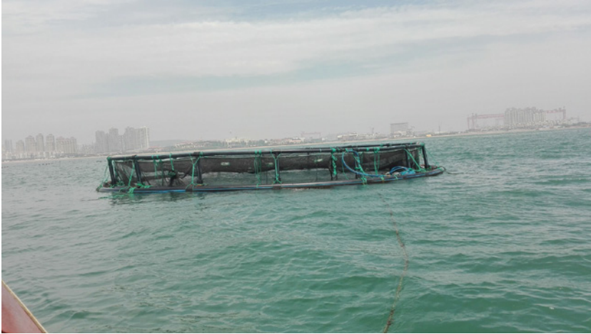
Figure 3.11.12 HDPE circular submersible cage.
