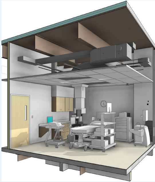
Figure 7-9 LOD 400 assembly Image courtesy of CannonDesign
