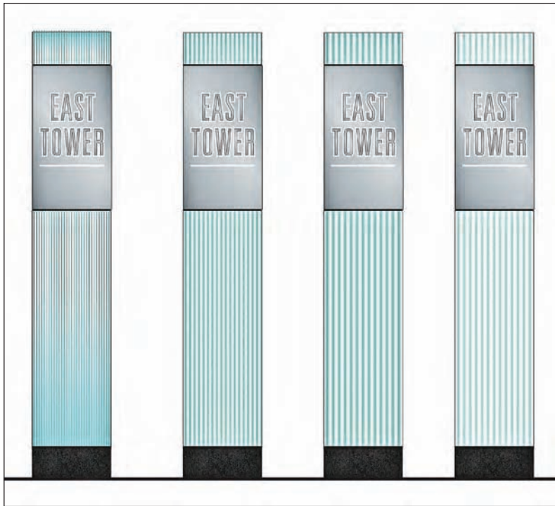
2.17 Design development phase: Study of glass rib size and spacing advances the design refinement of the pylon signs.
