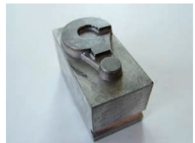
5.2 A piece of metal type. Metal type, now obsolete after five centuries of use, formed the basis for the currently used typographic measurement system.
