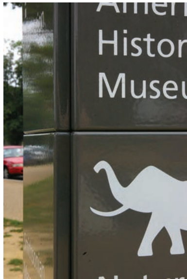
5.68 Porcelain enamel provides excellent durability for exterior signs, such as this sign on the National Mall in Washington, DC.
