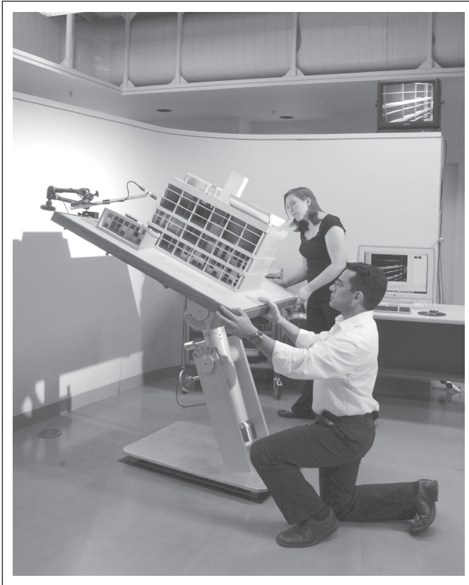
FIGURE 6.3 The Heliodon. This device uses a light source and a physical model to simulate the effects of sunlight on a building. This process allows architects to determine during the design phases how a building will function with respect to daylighting, shading, and shadows and to identify opportunities for energy savings.
