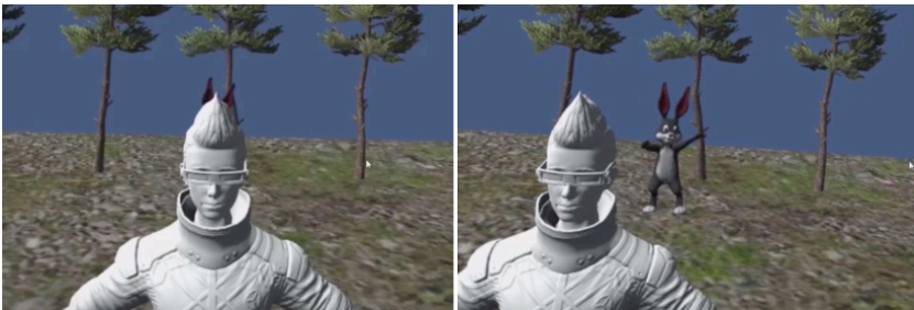
Figure 5.3. Parallax, illustrated here by the relative movement of one object with respect to others, through a simple lateral translation of the camera. For a color version of this figure, see www.iste.co.uk/arnaldi/virtual.zip
