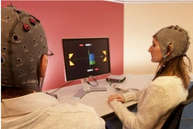
Figure 5.5. The multi-player BCI game “BrainArena”: both players are fitted with EEG helmets and can score goals to the left of right together, or can play against one another, by imagining movements of the left or right hand
