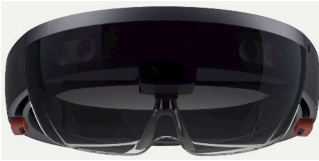
Figure 4.1. The Microsoft HoloLens augmented reality headset (© Wikimedia)
