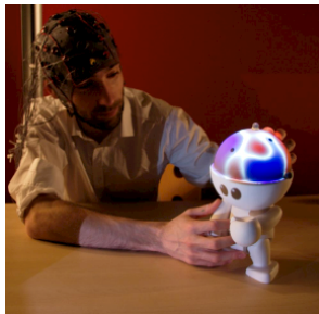
b) Teegi [FRE 14]: interaction with a physical representation of our brain activity
