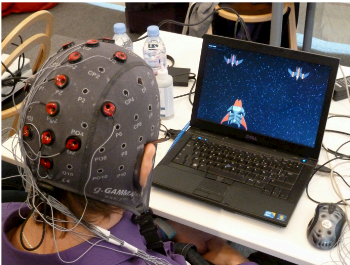
Figure 5.4. MindShooter , a video game inspired by the famous Japanese game “Space Invaders” and controlled here by a reactive BCI using SSVEP [LEG 13]
