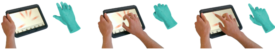
Figure 3.22. Illustration of an interaction technique called the "Thing" that uses a tactile tablet in order to capture the movements of the hand and animate a virtual hand [ACH 15]
