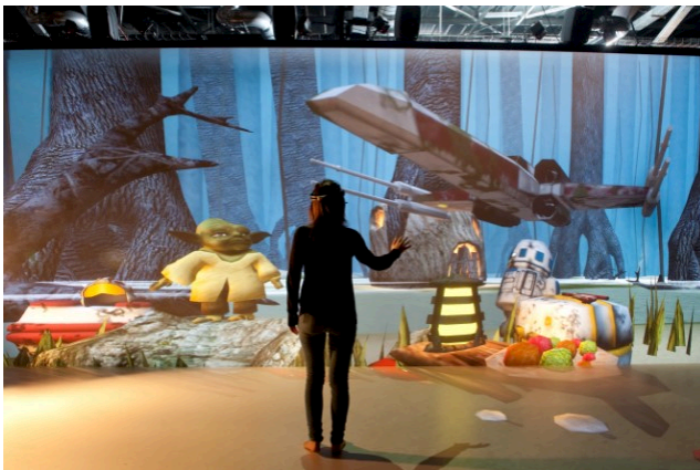
Figure 5.6. The VR application “Virtual Dagoba”: the user is fitted with a wireless EEG helmet and is immersed in an immersion room (Immersia, IRISA/Inria, Rennes) and a 3D scene inspired by the universe of the “Star Wars” films. The user can take the spacecraft up by concentrating (or bring it down by relaxing). For a color version of this figure, see www.iste.co.uk/arnaldi/virtual.zip
