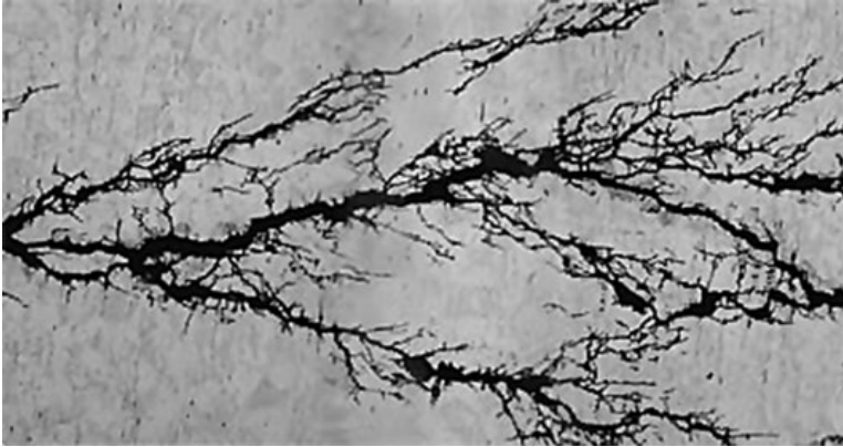
Figure 5.5 Stress corrosion versus general corrosion. Source: Reproduced with permission of NASA.
