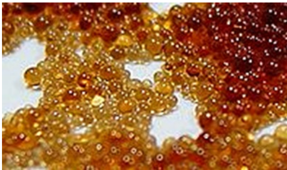
Figure 11.14 Typical ion exchange polymer bead. Source: Bugman, https://commons.wikimedia.org/wiki/File:Ion_exchange_resin_beads.jpg . © Wikipedia.
