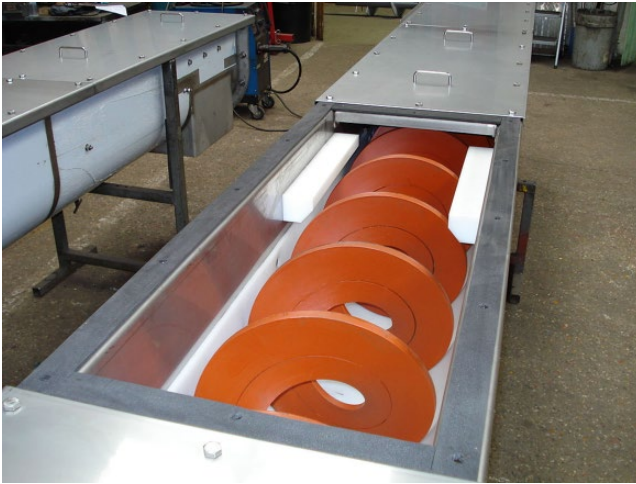
Figure 15.3 Operating screw conveyor. Source: https://commons.wikimedia.org/w/index.php?curid=9515471 . Used under CC BY 3.0 https://creativecommons.org/licenses/by/3.0/deed.en . © Wikipedia.
