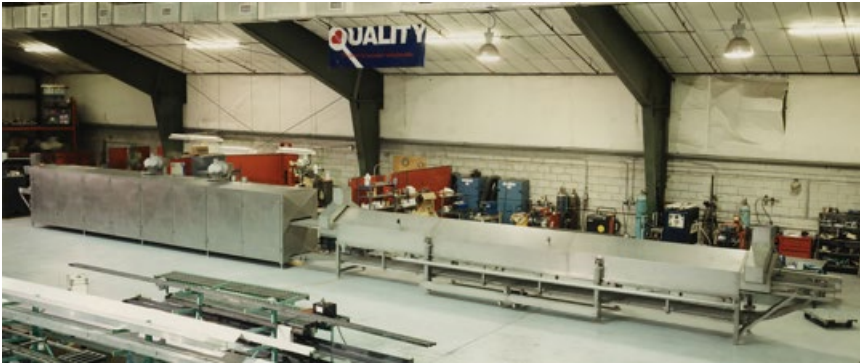
Figure 14.6 Food belt dryer. Source: https://commons.wikimedia.org/wiki/File:DEMACO_DTC-1000_Treatment_Center_for_Fresh_Pasta_Production_(April_1995)_003_crop.jpg . Used under CC BY-SA 4.0, https://creativecommons.org/licenses/by-sa/4.0/deed.en . © Wikipedia.
