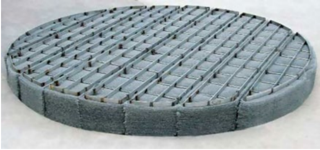
Figure 11.5 Typical demister. Source: Courtesy of Sulzer AG.
