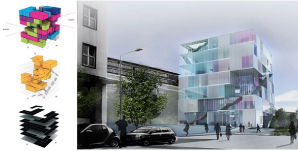
Figure 3.2. LAVA VOxEL extension for the architectural school in Stuttgart, 2009. Three diagrams (left) show the generative principles: 1) attribution of functions; 2) cell stacking and 3) distribution of the program. For a color version of the figure, see www.iste.co.uk/marsault/architecture.zip
