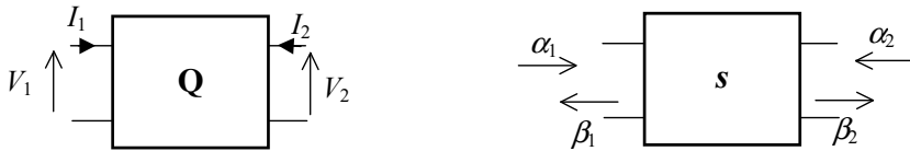
Figure 2.11. Representations of a quadripole, including currents, voltages and complex parameters on the left and using incident and reflected waves, and s -parameters on the right
