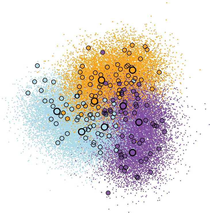
Figure 14.1 Test and training data generated by R code in this section. The data are colored by class. Test data are plotted as tiny points, training data are plotted as medium points with black boundaries, and the nine Gaussian means are plotted as large points with black boundaries.
