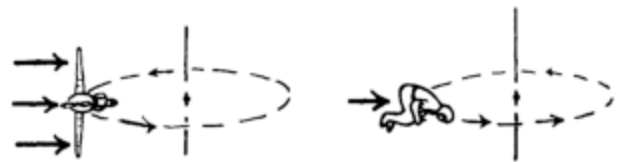
FIG. 21-20b. Air exerts forces on wings and body, pushing plane towards center of circle, in loop or turn. (In this sketch, gravity is ignored. In sharp turns it is relatively unimportant.)
