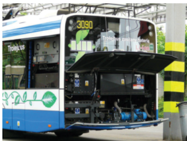
Fig. 5.14. Rear part of a Solaris Trollino 12 trolleybus, 3 battery modules (black boxes) and the charging system (a grey box in the upper part of the apparatus) are visible
