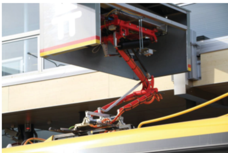
Fig. 2.4. Pantograph of charging system system Opp Charge (Tusku, Helsinki)
