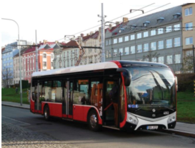
Fig. 2.6. Electric bus charged in two pole system (Prahá, Czech Republic)
