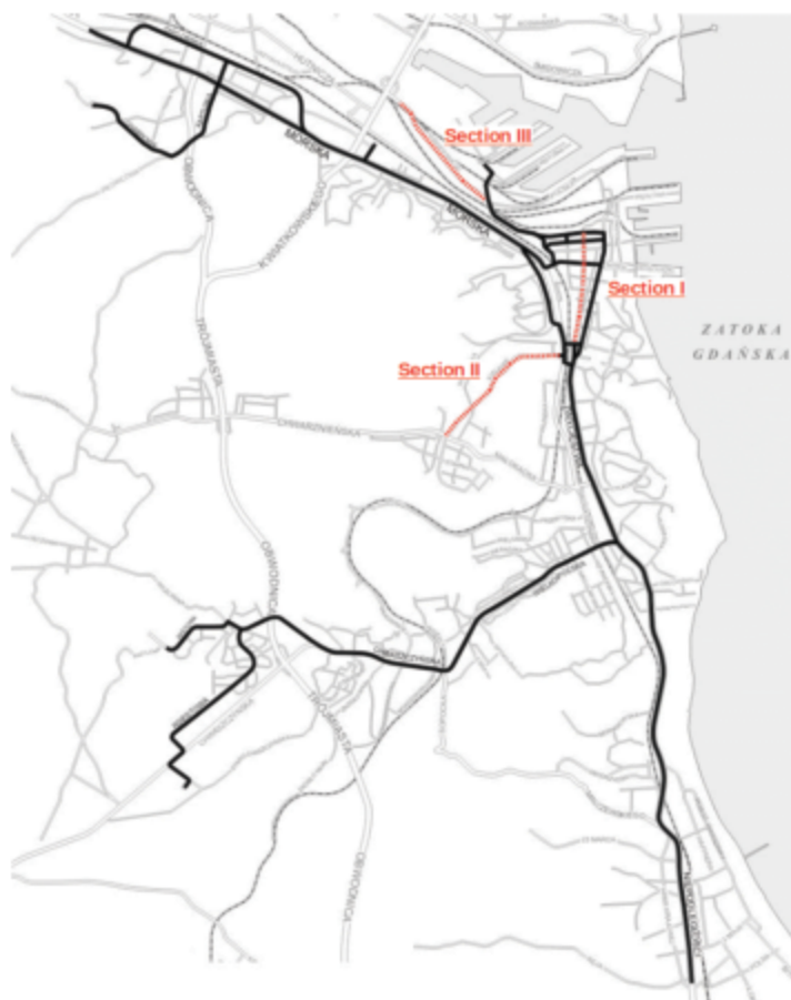
Fig. 7.3. The possibilities (red lines) of extensions of existing (black line) trolleybus network in Gdynia
