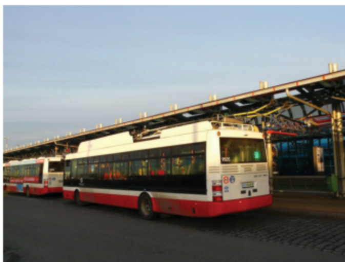
Fig 3.6. Trolleybus SOR TNB 12 on Letňany terminus in autonomous drive mode
