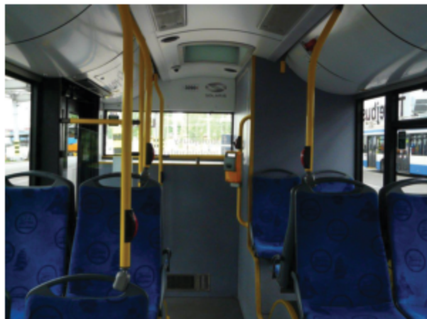
Fig. 5.15. Interior of the rear part of a Solaris Trollino 12 trolleybus. The vertical casing containing battery modules is visible
