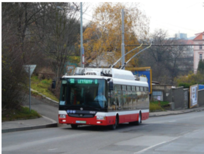
Fig. 3.4. Trolleybus SOR TNB 12 goes uphill on Prosecka street in Prague powered from the traction network
