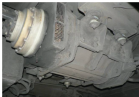
Fig 4.20. Trolleybus traction motors, the elements of second level insulation are visible
