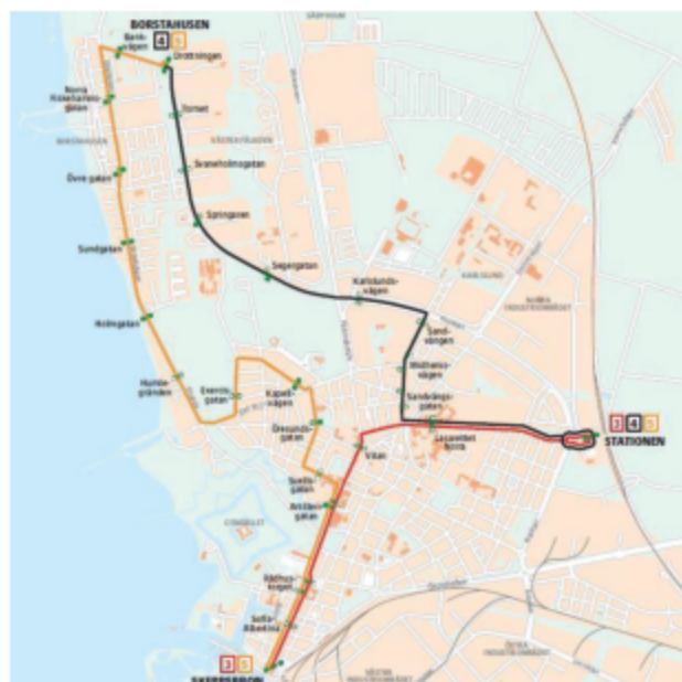
Fig. 3.1. Trolleybus system in Landskrona, line 3 - standard trolleybus line, lines 4 and 5 - battery operation [33]
