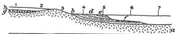
FIGURE 49. Diagrammatic section to illustrate unconformities and their effect on ground-water conditions. a to h are formations in the order of their age, a being the oldest and h youngest. b , d , and g are aquifers. Unconformities exist between a and overlying formations and between f and underlying formations. b , d , and g are aquifers. Problems: What will be the result of drilling at localities 1, 2, 3, 4, 5, 6, and 7, and to what extent are these results determined by the unconformities?
