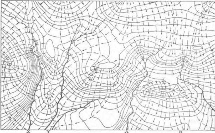
FIGURE 43. Diagrammatic map showing the form of the water table by means of contours (continuous lines), and directions in which the ground water moves (arrows) from intake areas to areas of discharge along the streams.
