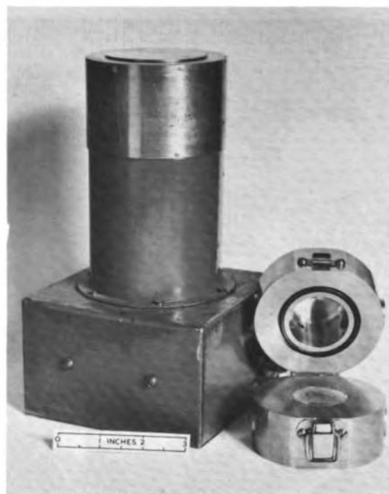
Figure 3. The 4\pi beta counter (open) and scintillation counter NaI(Tl) used at N. P. L. for 4\pi beta-gamma coincidence measurements of disintegration rate.
