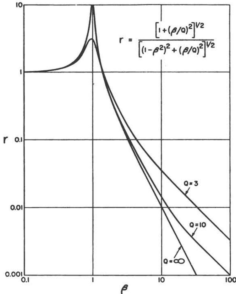
Figure 3 - Theoretical transmissibility of an ideal system consisting of a rigid mass, a massless spring in parallel with a viscous damper, and an infinitely rigid foundation. (After Plunkett)
