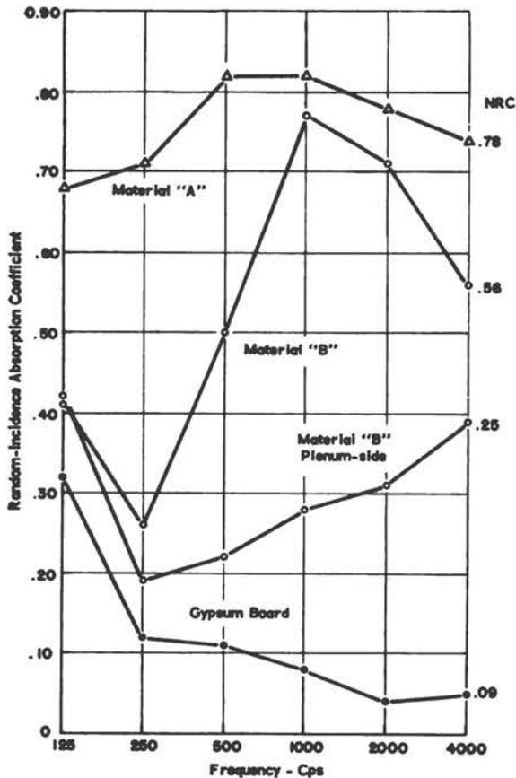
Fig. 3 - Reverberation-Room Absorption Coefficients, Simulated Suspended Ceilings, #7 Mounting - 10" Airspace
