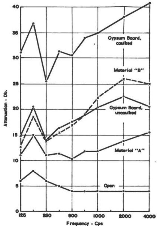
Fig. 4 - Reverberation-Room Transmission Spectra, Simulated Ceilings in Eastern System.
