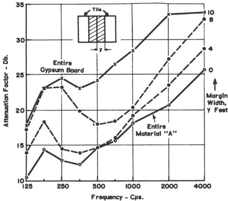
Fig. 6 - Attenuation Spectra, Material "A" vs. Gypsum Board Margin, 30" Plenum
