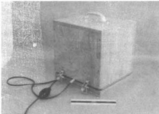
Fig. 1 - This box is similar to the one used for the demonstrations, except that the sound absorbing inner box is made of glass fiber blanket with a perforated metal cover, rather than used rug cushion, and the pad on which the noise maker rests is glass fiber material rather than rubberized hair.
