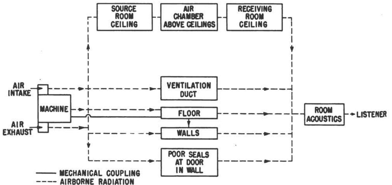
Figure 2 - Block diagram of noise transmission paths of Figure 1.
