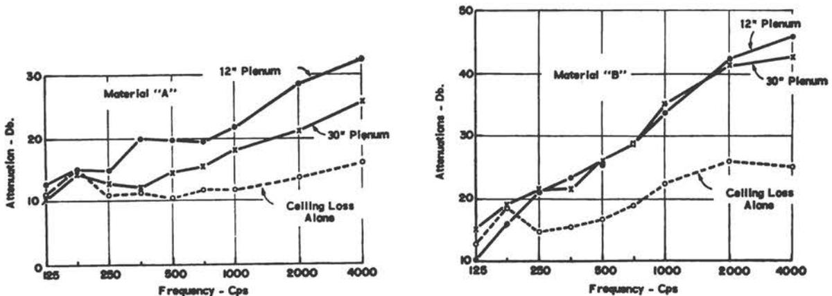
Fig. 7 - Two-Room Attenuation Spectra Compared to Transmission Loss
