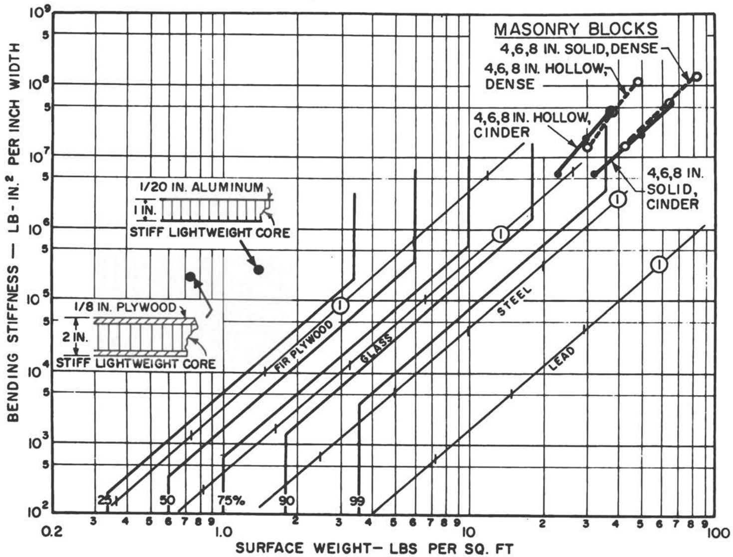
Fig. 3 - Approximate values of stiffness and weight for two lightweight-core panels and some masonry blocks.
