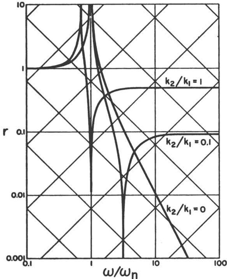
Figure 5 - Theoretical isolation provided by a vibration mount of stiffness  $k_2$  isolating a machine from a base having a stiffness  $k_1$ , in terms of the ratio  $k_2/k_1$  and normalized frequency. (After Plunkett)
