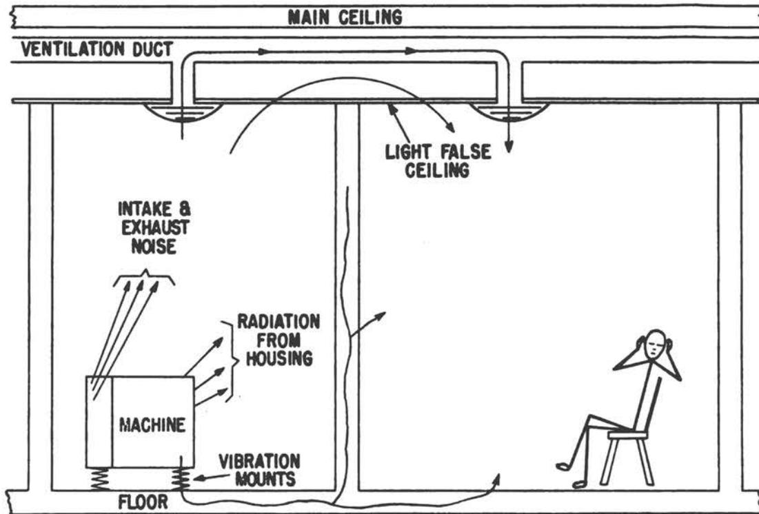
Figure 1 - Two adjacent rooms with noisy machine in one. Typical acoustic and vibration paths are indicated.
