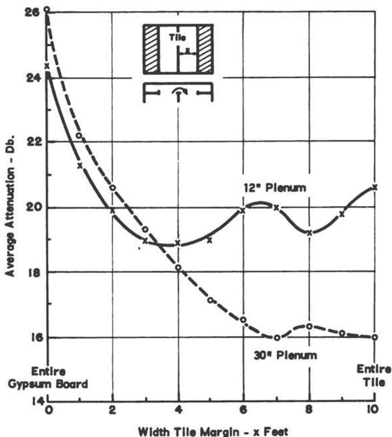
Fig. 5 - Average Attenuation vs. Margin Width, Material "A" Tile.
