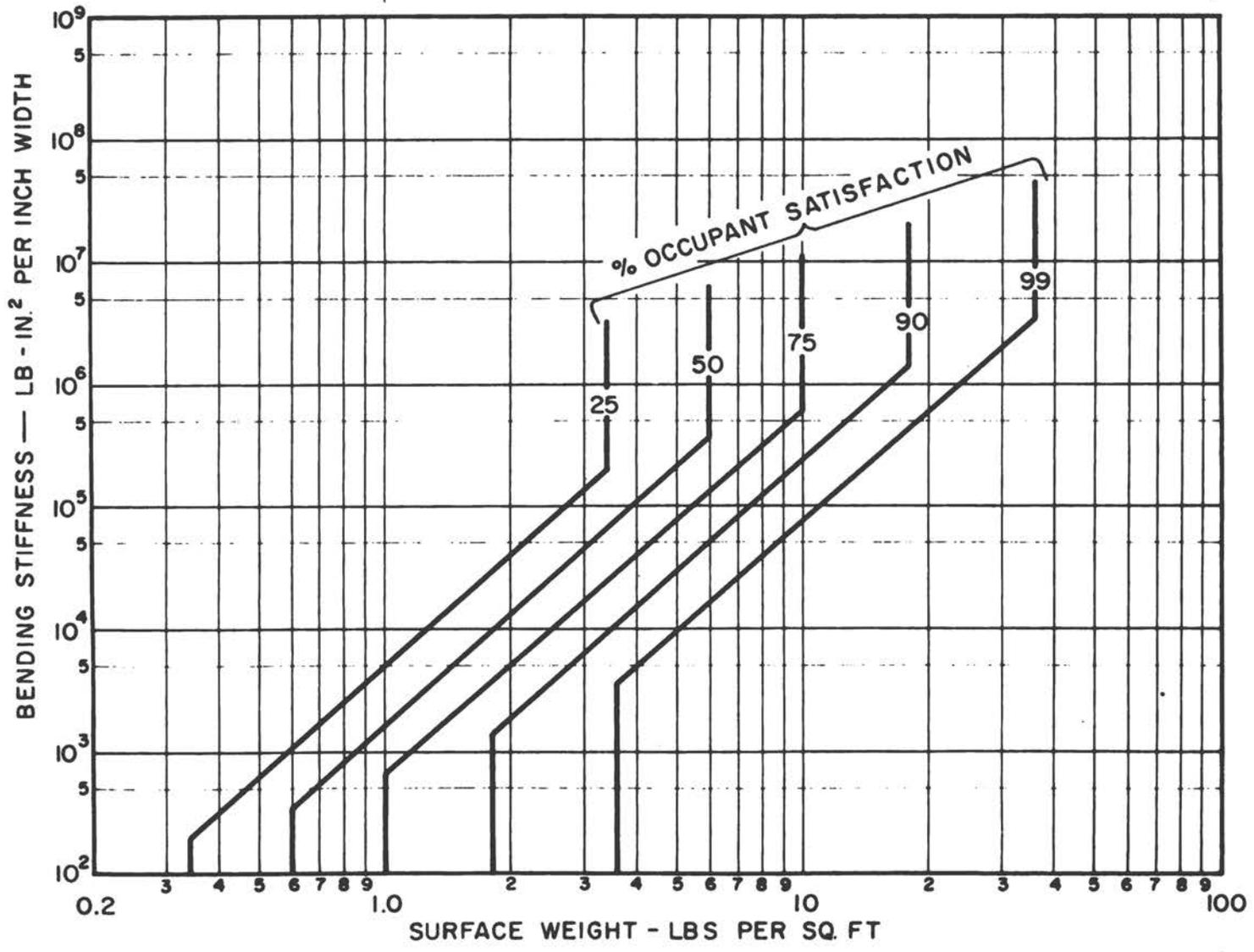
Fig. 1 - Approximate degree of speech privacy for walls with the indicated surface weight and bending stiffness, for one, typical, between-office situation.
