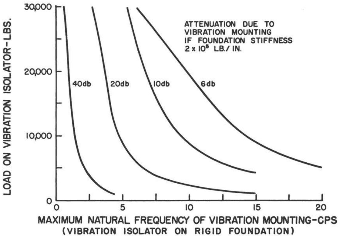
Figure 6 - Effect of load and natural frequency on the attenuation of a vibration mount, assuming foundation stiffness to be  $2 \times 10^5$  lb/in.
