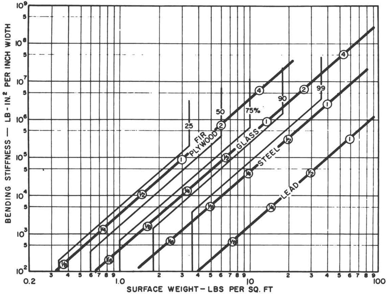
Fig. 2 - Approximate values of stiffness and weight for various thicknesses of solid panels. The circled numbers give the thickness in inches.
