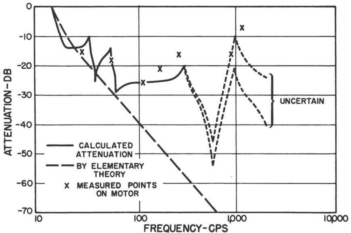
Figure 7 - Predicted values, in decibels, of vibration reduction using both elementary theory and actual mobility calculations. Measured values of attenuation are also indicated. (After Plunkett)
