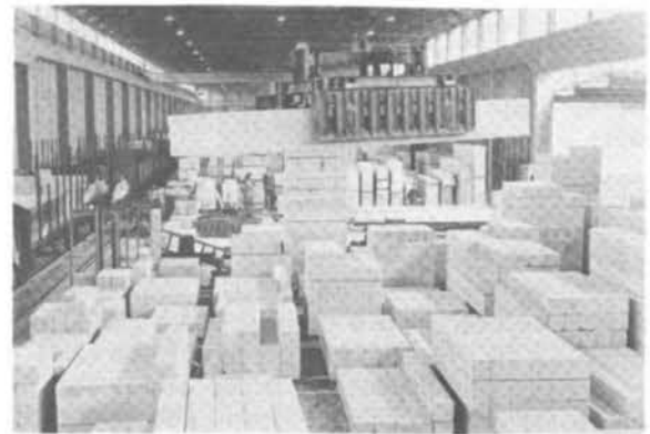
Fig. 2 - Cured autoclaved cellular concrete in Swedish factory showing lintels, beams and slabs.
