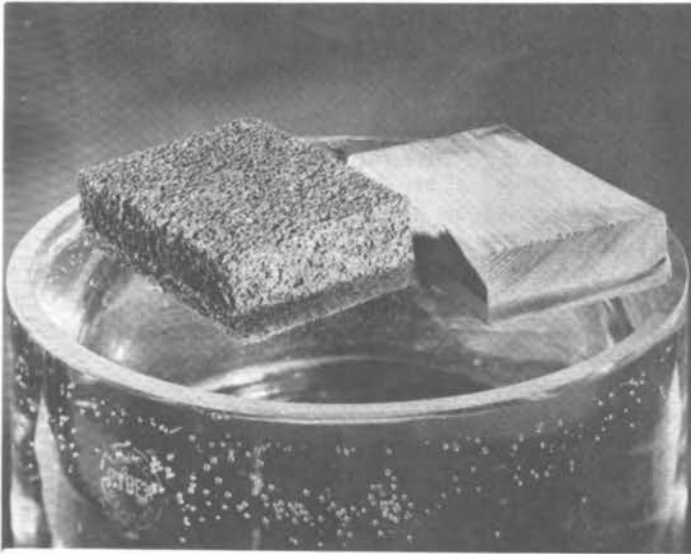
Fig. 1 - Foamed aluminum closed cell structure in water.
