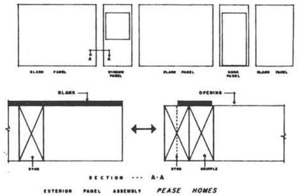
Fig. 6. Exterior panel assembly
