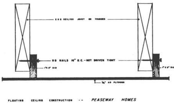
Fig. 5. Floating ceiling construction
