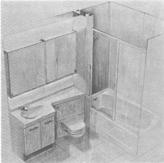
Fig. 2. Preassembled lavatory, wall-hung water closet and cabinet component.
