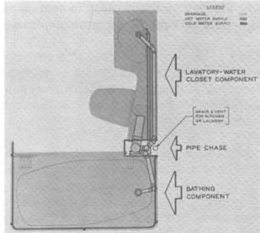
Fig. 3. Preassembled supply and drainage installed within cabinet structure.
