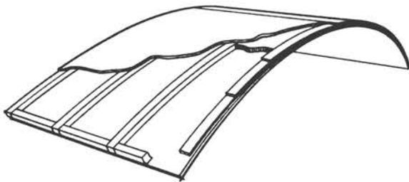
Fabrication - Because gluing is involved, box beams must be fabricated under close control. This usually eliminates fabrication in other than factory conditions.
