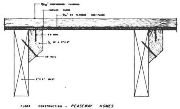
Fig. 4. Floor construction
