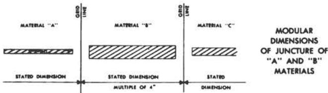
Fig. 2. Joining of two different modular materials.
