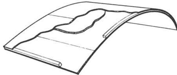
Fig. 5. Ribbed type curved panels.
