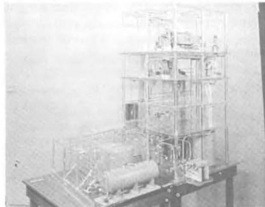
Fig. 7. Completed true-scale piping model with all phases such as electrical and mechanical shown.
