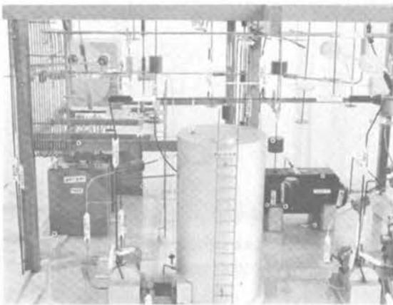
Fig. 6. Typical fine wire model of a process unit.
