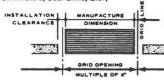
NOTE: In General, modular units, components or assemblies should have no integral elements extending beyond the "grid opening.
