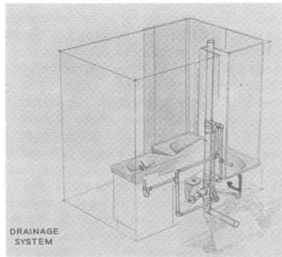
Fig. 5. Supply and drainage for tub-shower component.
