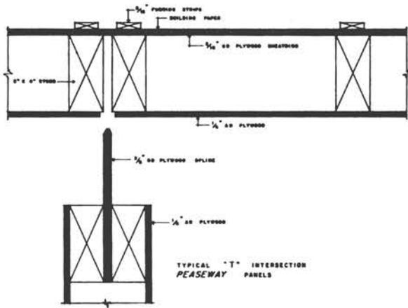
Fig. 3. Typical "T" intersection
