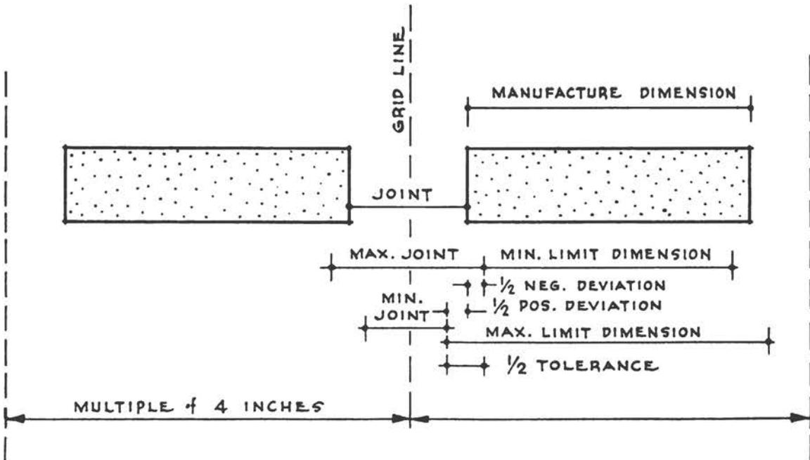
Fig. 3. Note drafting convention designating dimensions to the grid line with an arrowhead and to the off-grid point with a dot.
