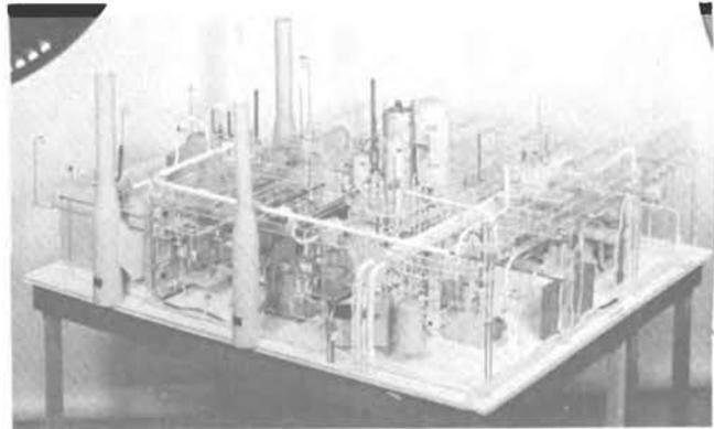
Fig. 5. Completed true-scale piping model with all phases such as electrical and mechanical shown.
