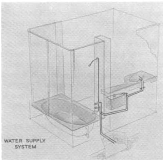
Fig. 4. Tub and walls to be added to lavatory-water closet component.
