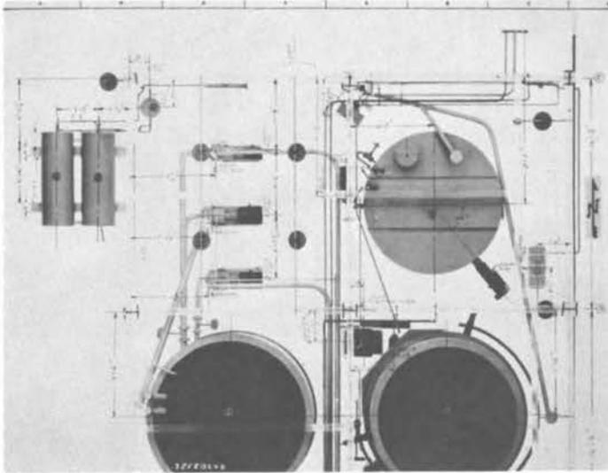
Fig. 8. A portion of a shadowless model photo-drawing.
