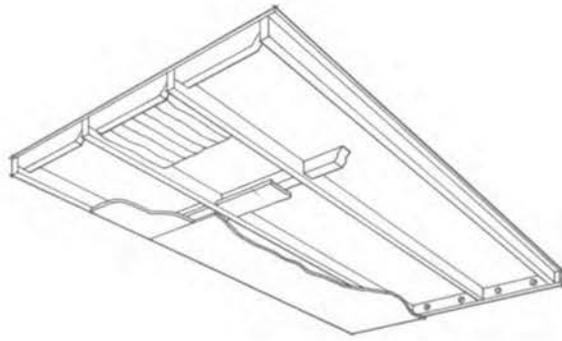
Fig. 4. Sandwich type curved panel.
