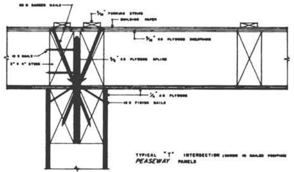
Fig. 2. "T" intersection nailed in place
