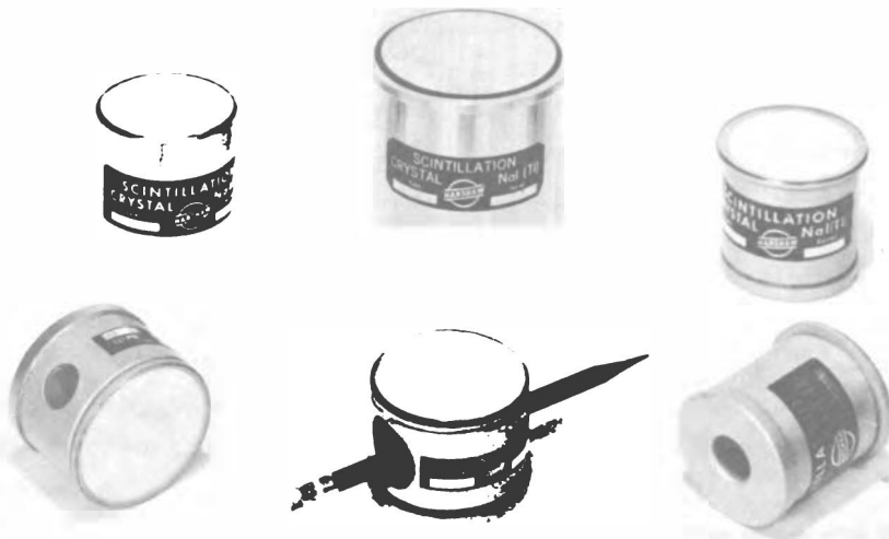
Fig. 6. Sealed NaI(Tl) crystal assemblies for a variety of applications. Transparent windows are provided for optical coupling to photo-multiplier tubes (Harshaw Chemical Company).
