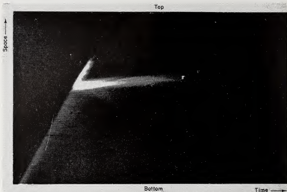
Figure 5. Same phenomena as Figure 4, but with 10 additional mg of powder. Extinction is obtained. Same luminosity and velocity reduction as in Figure 4 are observed.
