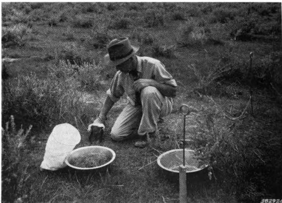
FIGURE 3. Clipping blue grama ( Bouteloua gracilis ) to determine herbage production. Upright strips have been welded to blades of grass shears to assist in collecting the herbage. The chain with the steel pin at both ends is a kind commonly used to circumscribe boundaries of circular plots.
