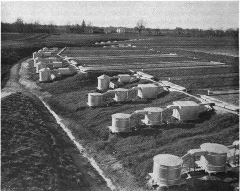
FIGURE 7. Permanent plots for studying runoff and erosion at a conservation experiment station. Below each plot is a silt box and one or more storage tanks. Between the box and tanks are divisors to take aliquot samples of the runoff. ( U.S. Soil Conservation photo NJ-R2-39 )
