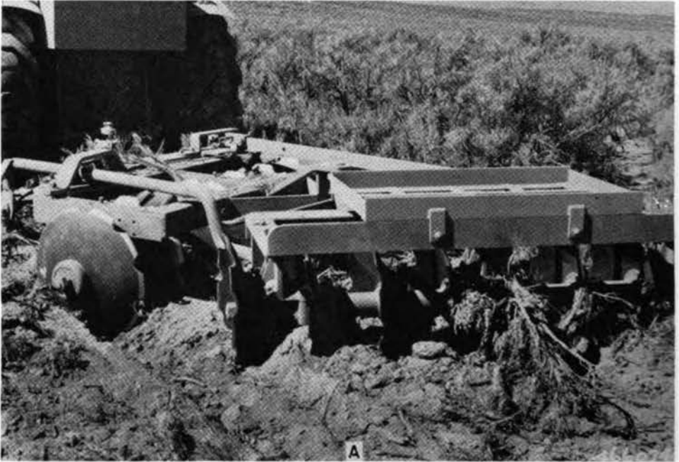
FIGURE 3. Four kinds of equipment commonly used on rough rangelands: A , heavy offset disc; B , brushland plow especially adapted to brushy and rocky terrain; C , beater used for reducing short stiff brush; and D , rail used to remove sagebrush. ( A , B , and D , U.S. Forest Service photos, and C , courtesy of the Caterpillar Tractor Company)
