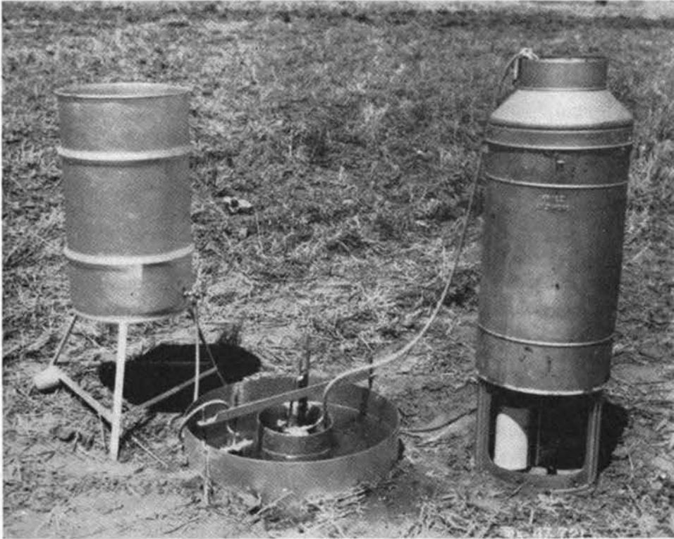
FIGURE 3. Concentric-ring type infiltrometer with automatic water supply recording gauge. The rings alone are frequently used with manual application and measurement of water. ( U.S. Soil Conservation Service photo )
