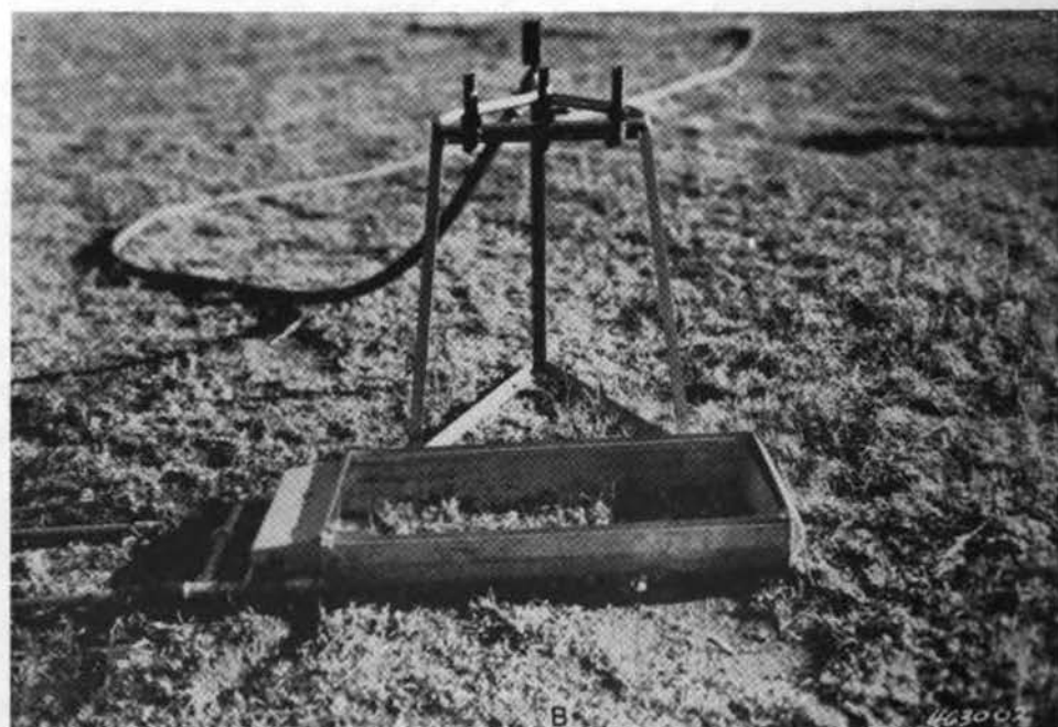
FIGURE 5. Rocky Mountain infiltrometer. A , in field use. B , closeup of apparatus. (U.S. Forest Service photos)
