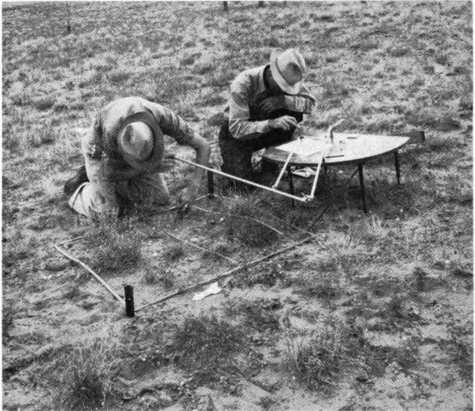
FIGURE 2. The pantograph used for charting quadrats. Two persons are required to chart the vegetation, one to identify and trace the vegetation and the other to handle the recording needle and make other records. ( U.S. Forest Service photo )
