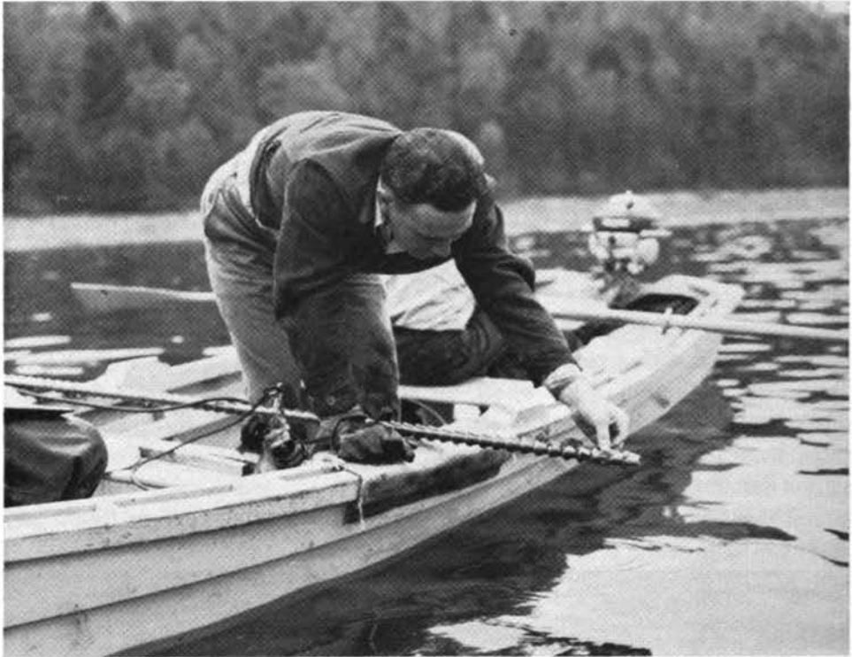
FIGURE 12. A spud is used to bring up samples of sediment from bottom of reservoir. (U.S. Soil Conservation Service photo NY-881)
