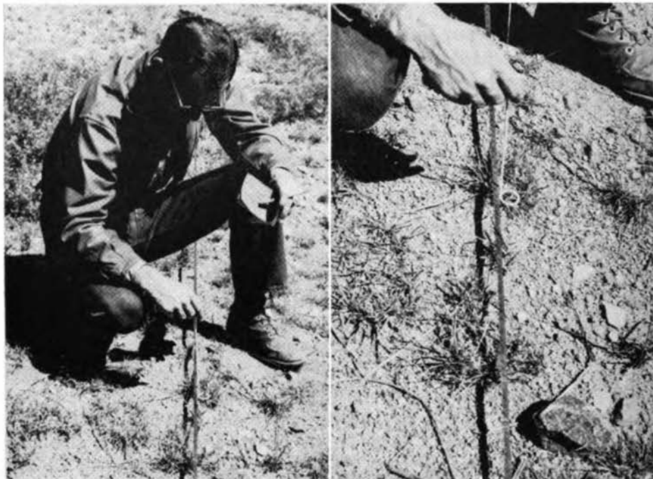
FIGURE 7. Method of using the \frac{3}{4} -inch diameter loop. One man makes the observations and records the data as to species, litter, bare ground, erosion pavement, and rock. Photo on right is closeup of wire loop showing an observation on a perennial grass.
