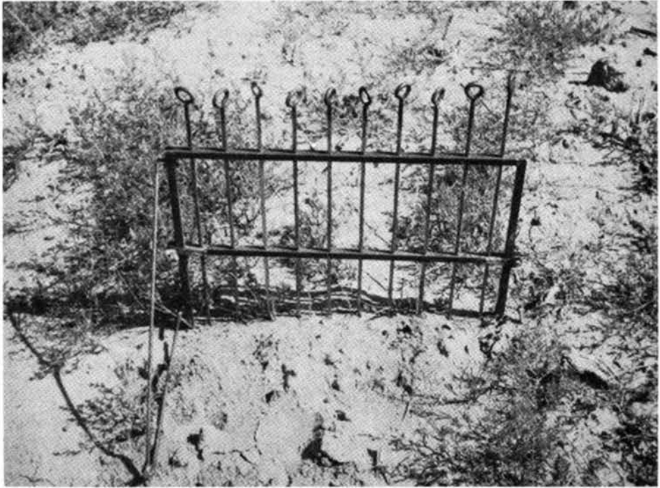
FIGURE 5. Apparatus used in the point method. Points can be held in vertical position as shown or at an angle of 45 degrees. ( Utah State University photo )
