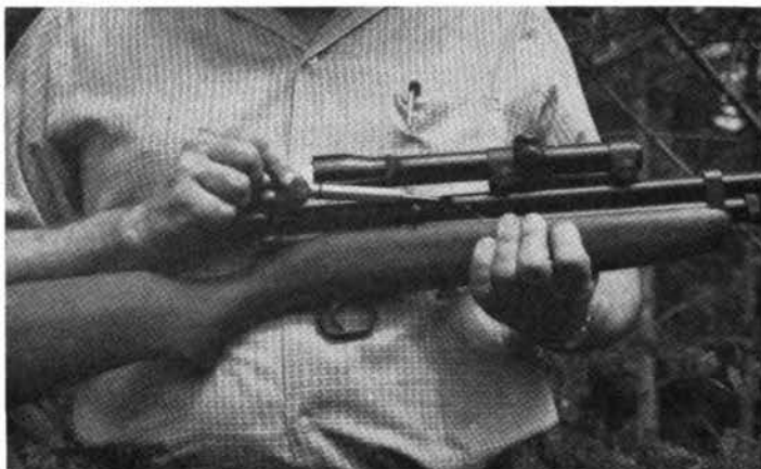
FIGURE 13. Air gun and dart used to capture deer for experiments. On contact the dart injects a paralyzing or stupefying drug. The dart is propelled by compressed carbon dioxide and is effective up to 40 yards. (Courtesy Lee A. Yeager)
