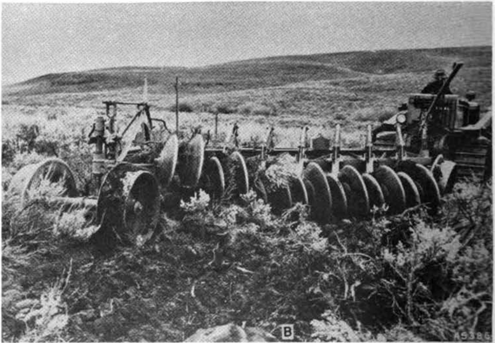
FIGURE 3. Four kinds of equipment commonly used on rough rangelands: A , heavy offset disc; B , brushland plow especially adapted to brushy and rocky terrain; C , beater used for reducing short stiff brush; and D , rail used to remove sagebrush. ( A , B , and D , U.S. Forest Service photos, and C , courtesy of the Caterpillar Tractor Company)
