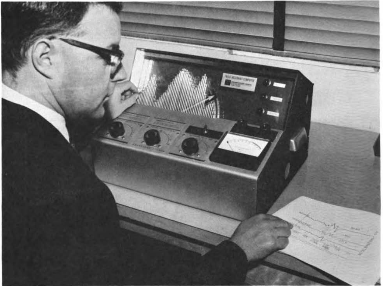
Figure 17. Prototype Computer Being Used to Assess the Effect of an Experimentally Measured Acceleration Input
