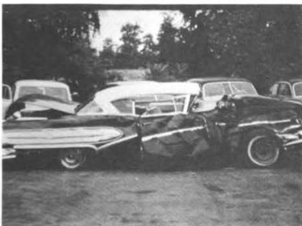
Figure 8. Vehicle was hit at right angle by southbound vehicle after crossing the median out of control.
