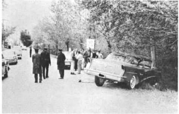
Figure 1. Vehicle shows a 24° swing to the left after hitting a tree at 40 m.p.h.
