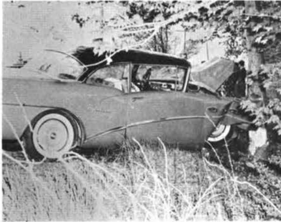
Figure 2. Impact site is at right-front headlamp. The collision course is the same as the point from which the photo was made.
