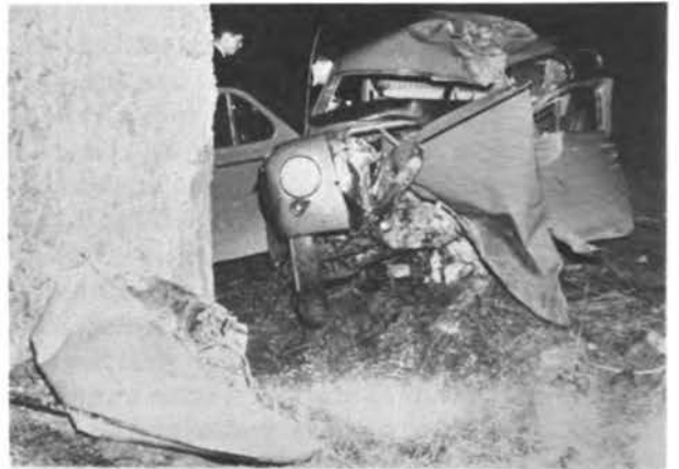
Figure 5. Results of a tree collision at 80 miles per hour. The driver was killed on the steering column. The right-hand passenger, wearing a lap belt and long stretching diagonal chest strap, had severe leg injuries due to the engine penetrating to the front seat, but had no head or chest injuries, and remained conscious after the impact.
