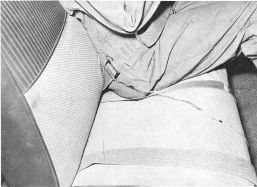
Figure 5. Belt Tensiometer Installation.
