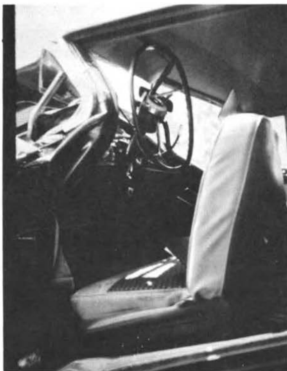
Figure 10. Steering wheel damage indicates path of body travel in hitting vehicle. (Figure 9)
