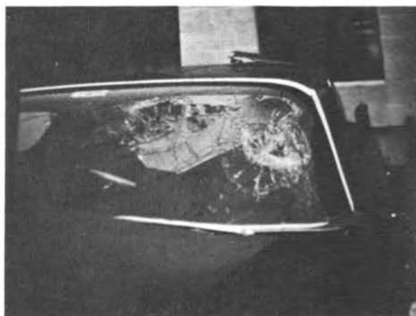
Figure 11. Two head impacts in windshield. On the driver's right is a passenger impact. On the driver's left is impact made by head of driver of car in Figure 8. This driver was essentially a missile.
