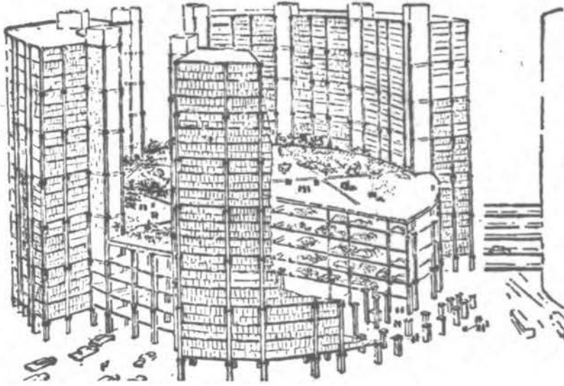
Figure 2. Center City designed by Louis Kahn, 1957. Circular buildings are "vehicular harbors or municipal entrance towers." Street level is used for markets; perimeter for hotels and offices; inner areas for parking and storage.
