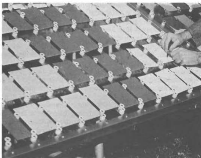
Figure 3 -- Knife adhesion testing of paint on panels exposed at the U. S. Steel Corporation site outside Pittsburgh, Pennsylvania.
