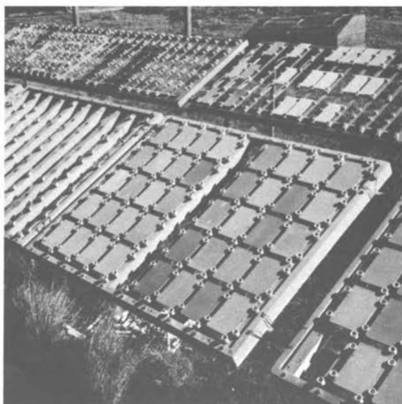
Figure 3 -- Typical exposure racks for test panels.
