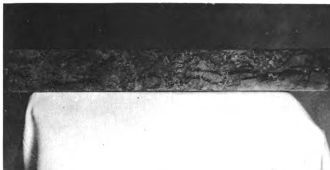
Fig. 4. Typical beam of undisturbed Boston blue clay frozen in horizontal position. Ice-lenses oriented horizontally, parallel to longitudinal axis of beam. Note magnets in ends of specimen
