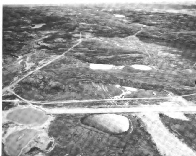
Fig. 4. Airstrip of station in Fig. 3. Note material pulled in from moraine. Road follows bare rock surface
