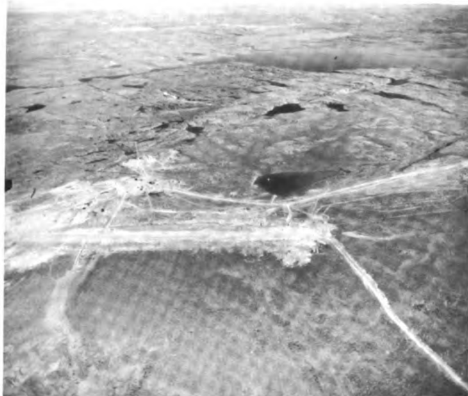
Fig. 2. Station in Melville Peninsula. Note development of airstrip on slope. Soil flow is indicated by striping
