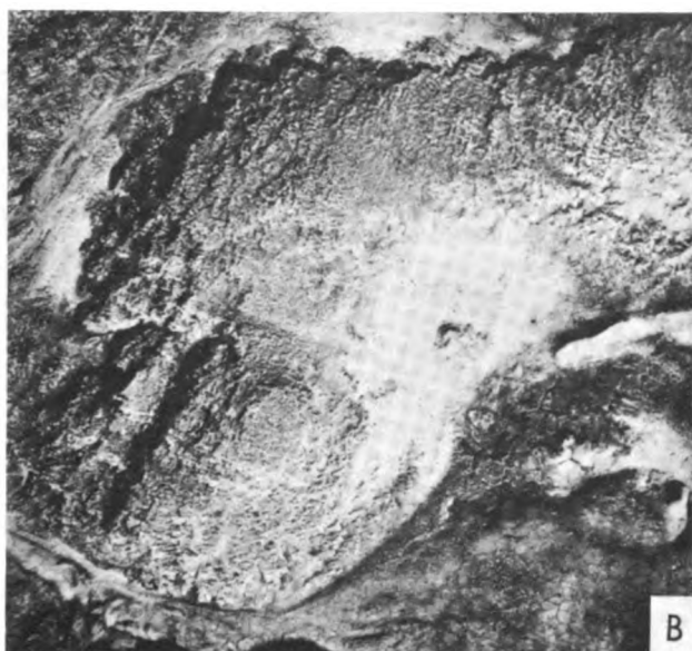
Fig. 3. Failure created when ditch was constructed over ice-wedges in jointed bedrock. These wedges can be predicted from the airphoto pattern of the area
