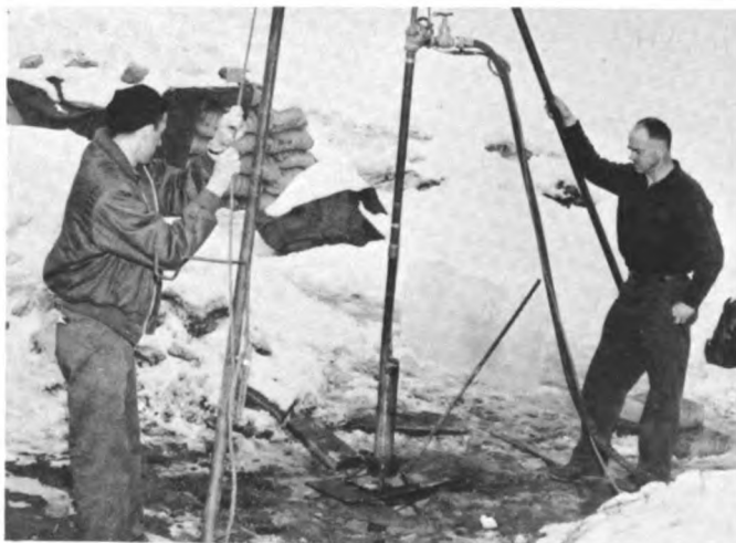
Fig. 1. Apparatus in place (KR#192) showing support tripod burner, bottom guide with removable cover plate in place, support rope, and flow control valves for air and fuel
