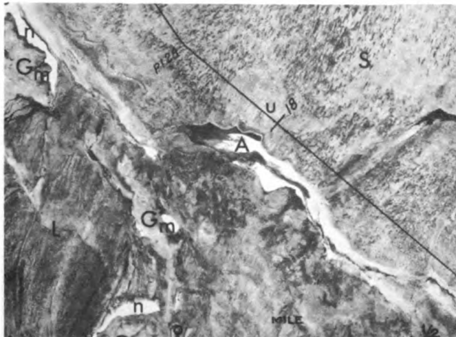
Fig. 4. Grade considerations necessitated following the base of this smooth hillside. Three isolated remnants of granular materials were mapped (Gm, see text) for field exploration and testing
