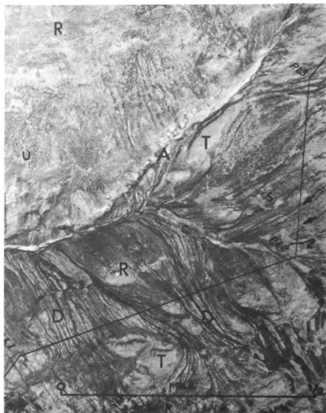
Fig. 2. Airphoto shows route location in vicinity of Mile 2. Letters are symbols for terrain conditions described in the text. Arrows point to localities of potential snowdrift. Grades are a major consideration in road location. Note distinctive gullies on terrain D
