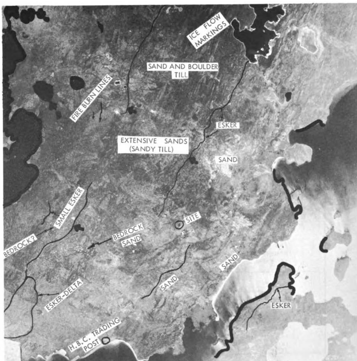
Fig. 6. Airphoto interpretation for construction materials in permafrost
