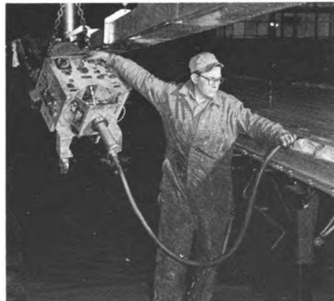
FIGURE 7 Insulating trailer with frothed foam.
