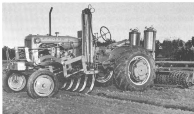
FIGURE 52 Tractor-mounted chisel-injection applicator. Cultipacker behind for sealing. (Courtesy of Shell Development Company.)
