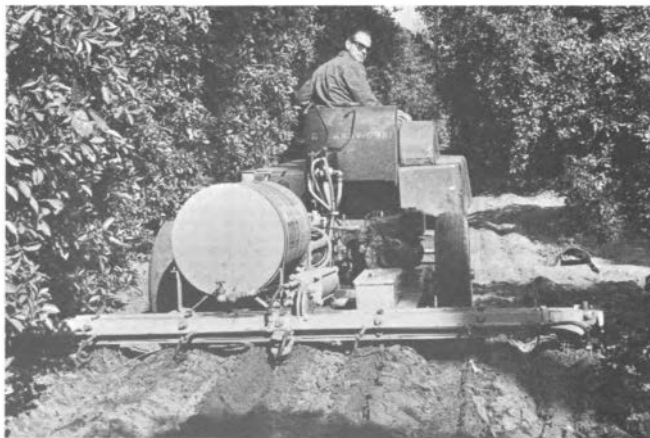
FIGURE 56 Side-dress of citrus by chisel injection of DBCP for control of citrus nematode ( Tylenchulus semipenetrans ). (Courtesy of the Department of Nematology, University of California, Riverside.)
