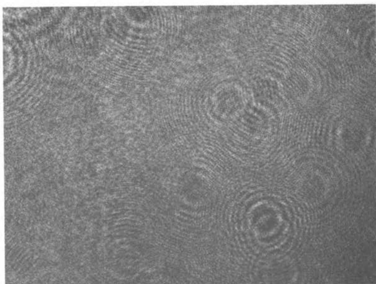
FIG. 2. A typical hologram. The visible pattern is caused by dust in the reference beam and it is not related to the image recorded on the hologram.
