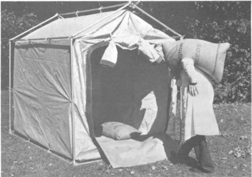
FIGURE 52 A portable–demountable tent for commodity and nursery-stock fumigation. (From Canada Department of Agriculture)
