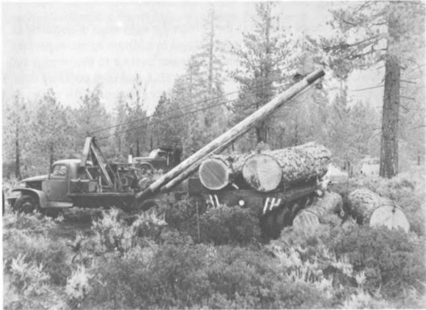
FIGURE 22 A mobile loader used in the sanitation-salvage logging of ponderosa pine to reduce losses caused by the western pine beetle. Infested trees and those considered most likely to be killed by the beetle in the near future are removed to reduce the beetle population and to improve the condition of the residual stand. Lassen National Forest (U.S.A.) (USDA photograph)
