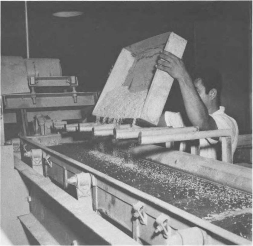
FIGURE 40 Mass rearing of screw-worms. The mature larvae are placed in trays of sawdust to pupate. Every 8 hours the trays are emptied onto a machine that screens out the sawdust. The pupae and any remaining larvae are then placed on a moving belt; pupae remain on the belt, but larvae are driven by lights to a collecting trough at the edge of the belt and are returned to the sawdust. (USDA photograph)
