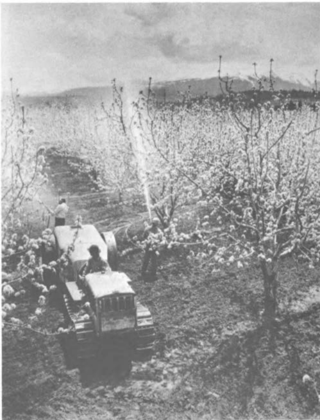
FIGURE 43 Hydraulic high-pressure, high-volume sprayer. (From John Bean Division, FMC Corporation)
