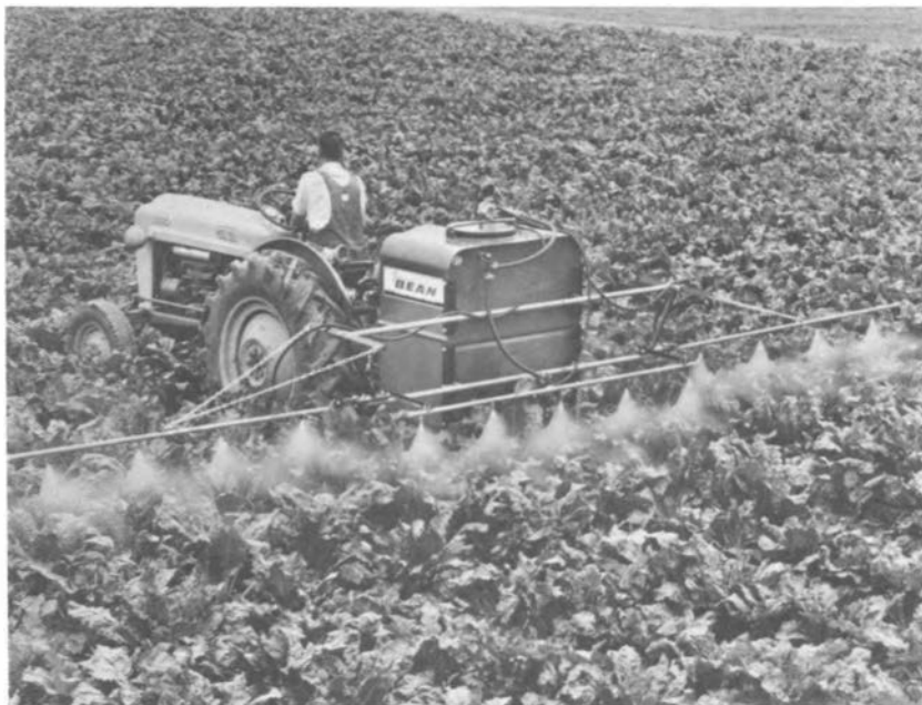
FIGURE 42 Hydraulic low-pressure, low-volume sprayer. (From John Bean Division, FMC Corporation)
