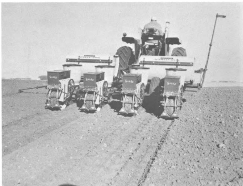
FIGURE 47 Granular-insecticide applicator mounted on a four-row planter. (From Gandy Company, Inc.)
