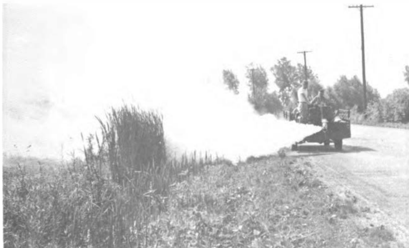
FIGURE 46 Aerosol generator or fogger. (From Michigan State University)
