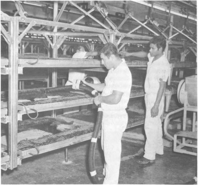
FIGURE 38 Mass rearing of screw-worm larvae in large vats. A mixture of ground meat, citrated beef blood, and water is piped into the vats and maintained at 37°C by electric heating elements below each vat. The racks containing the vats move along a monorail. (USDA photograph)
