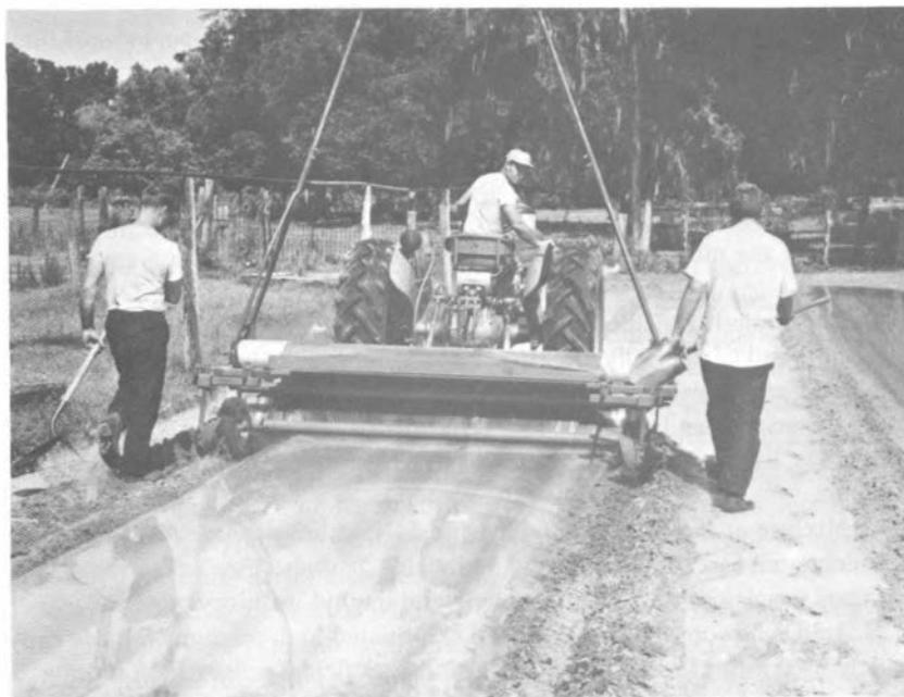
FIGURE 55 Soil-fumigant applicator with a device for laying plastic film to seal in highly volatile fumigants. (From The Dow Chemical Company)
