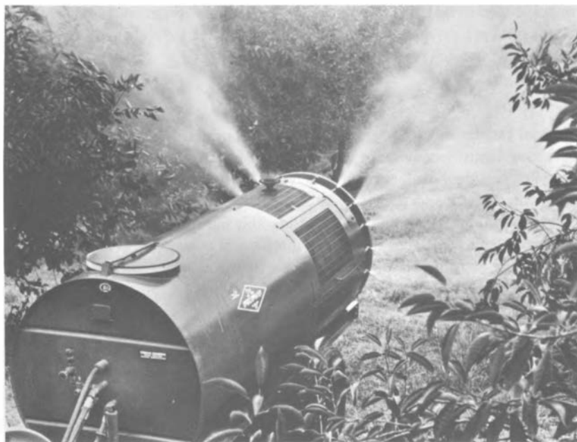
FIGURE 44 Air-blast sprayer. (From John Bean Division, FMC Corporation)
