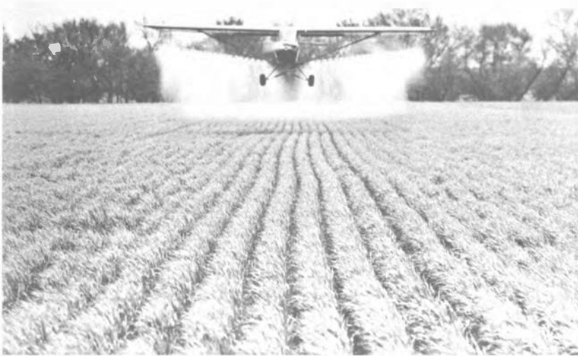
FIGURE 48 Fixed-wing airplane with boom-type sprayer. (From Michigan State University)
