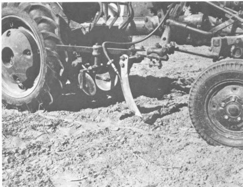
FIGURE 56 Soil-fumigant applicator for row treatments with low-vapor-pressure fumigants. (From The Dow Chemical Company)
