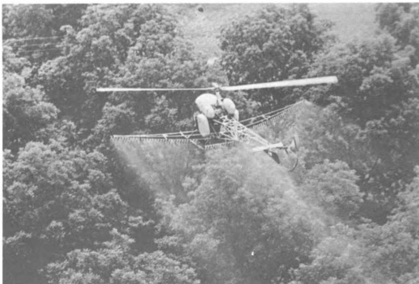
FIGURE 49 Helicopter with boom-type sprayer. (From Bell Helicopter Company)
