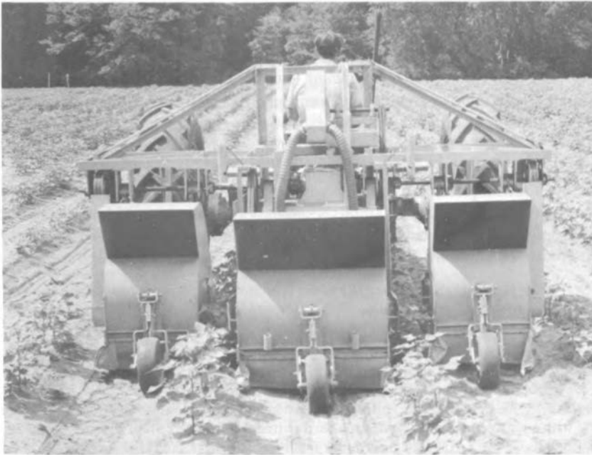
FIGURE 33 Flail machine designed to collect and destroy fallen cotton squares for boll weevil control.
