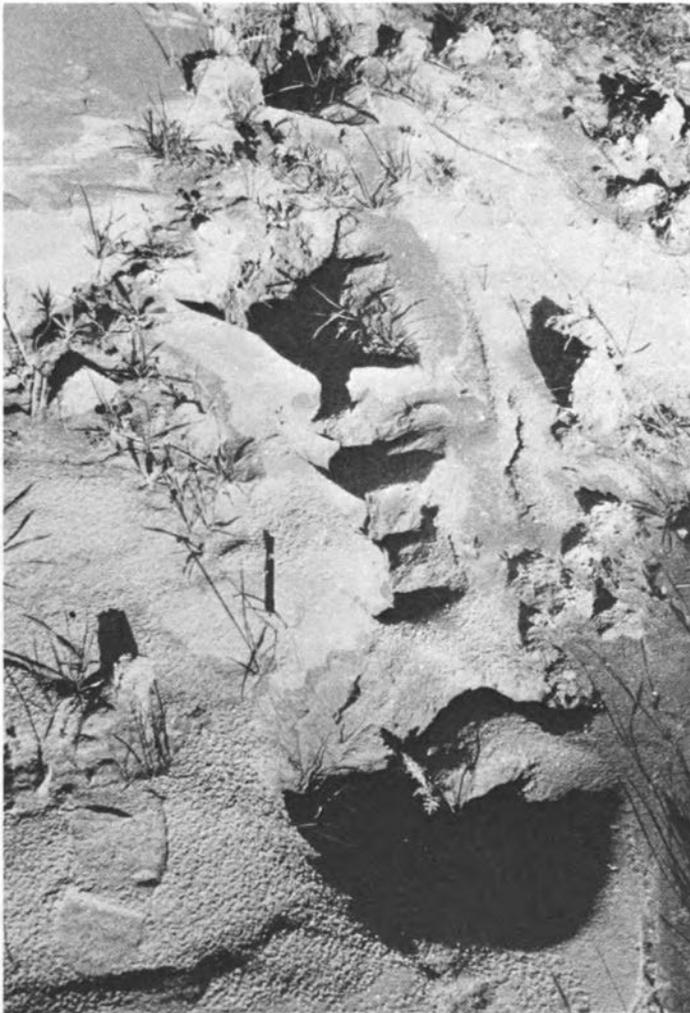
**Figure 31.** Detail of the sandboils shown in Figure 30.
