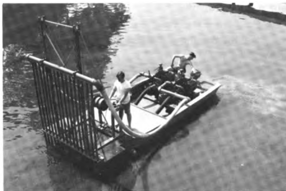
FIGURE 3 Hydraulic-jet device for uprooting submerged aquatics. (Photograph courtesy of D. Talbott, Annapolis, Maryland.)
