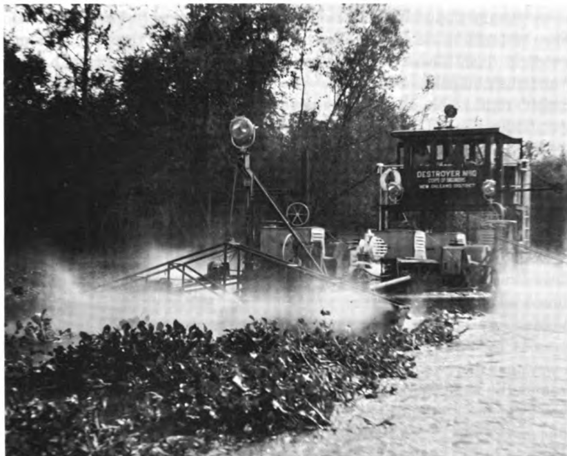
FIGURE 7 "Sawboat"-type unit for destroying water hyacinths shown in action. (Photograph courtesy of U.S. Army Corps of Engineers, New Orleans District.)
