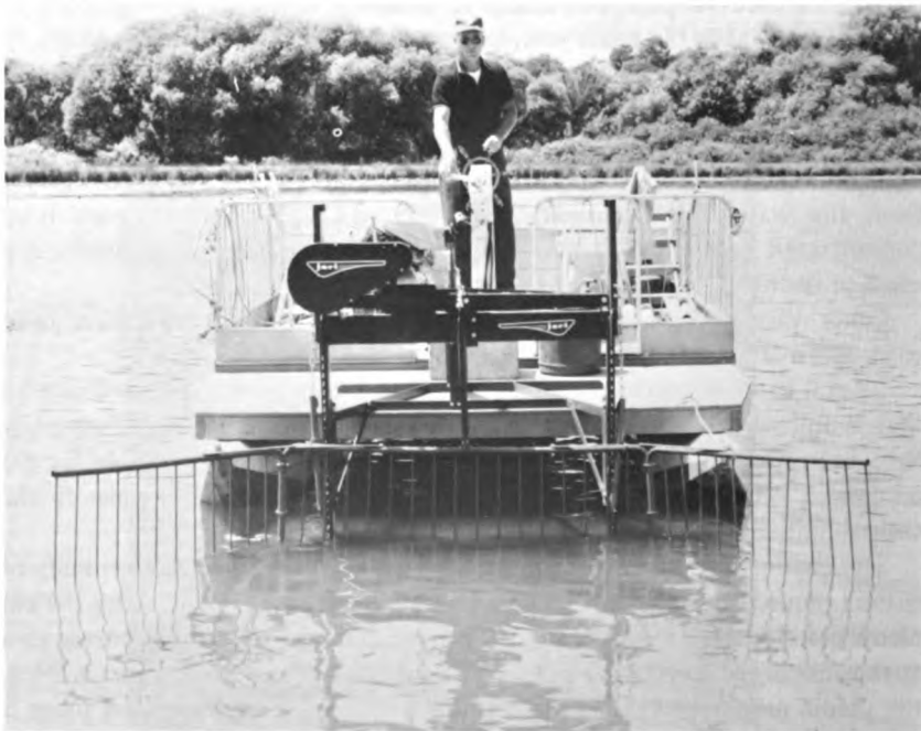
FIGURE 4 Underwater mower and weed rake. Rake is mounted in front of small mower on bow of pontoon boat. (Photograph courtesy of Jari Products, Minneapolis, Minnesota.)
