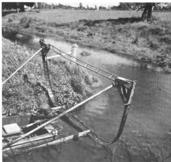
FIGURE 2 "U"-shaped reciprocating mower drawn behind boat. (Photograph courtesy of B. Powell, Christchurch, New Zealand.)
