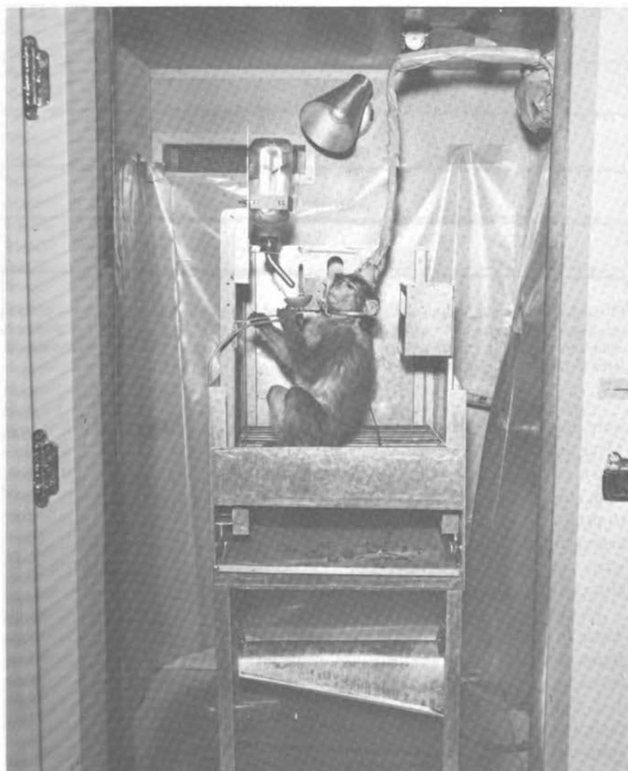
FIGURE 1 Rhesus monkey in recording chamber. Surgically implanted electrical connector mates to cable and to implanted sensors for recording brain temperature, electroencephalogram, electromyogram, and electrooculogram. Each animal was studied for 2 to 3 days in this booth after spending at least one postoperative month in a room with light from 0800 to 2000 hr, alternating with darkness.
