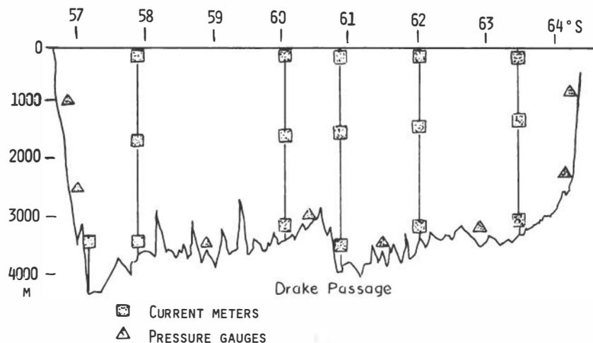
FIGURE 3.3 Recommended eventual arrangement of instruments across the Drake Passage; the first long-term moorings would involve fewer instruments.
