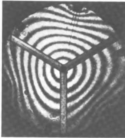
FIGURE 9 Mirror deflection contours, three-point support.
