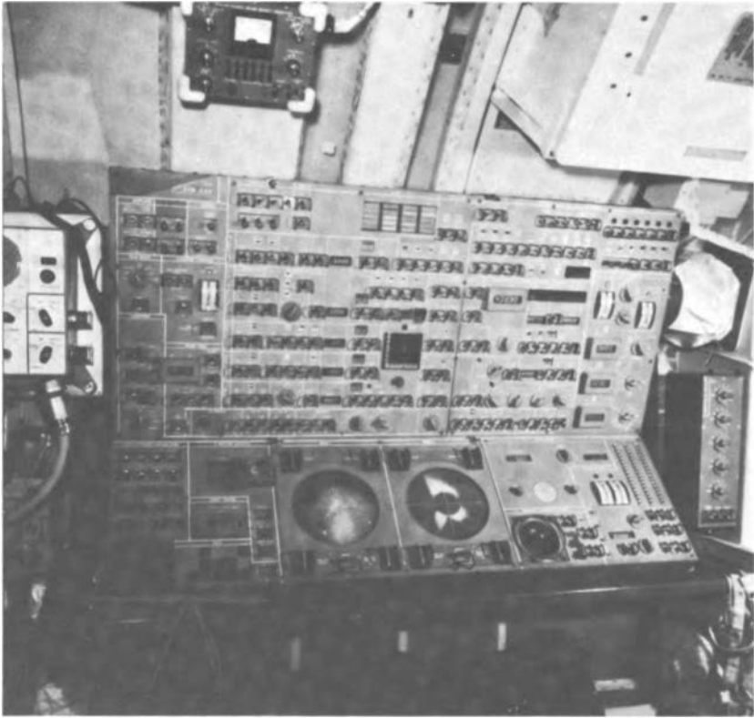
FIGURE 3 The ATM control and display panel mounted in the MDA. (NASA photo.)
