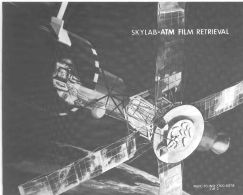
FIGURE 2 A view of the ATM during a film-retrieval EVA. The astronaut seen at the solar end of the canister is retrieving film from the xuv spectroheliograph and uv spectrograph. Film from the other experiments is retrieved through the door visible in the upper side of the ATM.
