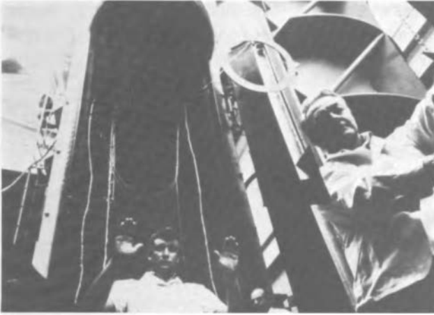
FIGURE 5 Side access vertical test tank.
