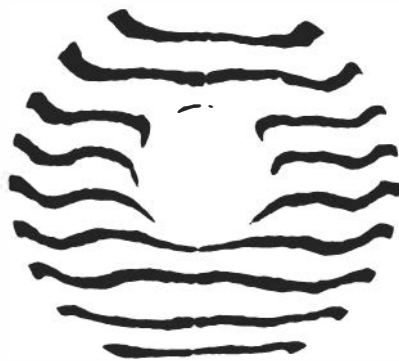
b. Test in autocollimation (double pass)
