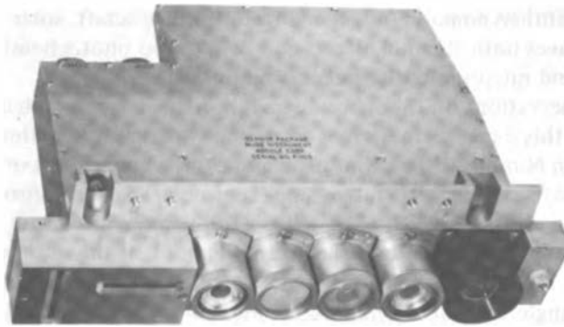
FIGURE 1 MUSE experiment sensor package with five sensors and digital solar aspect sensor at the top.
