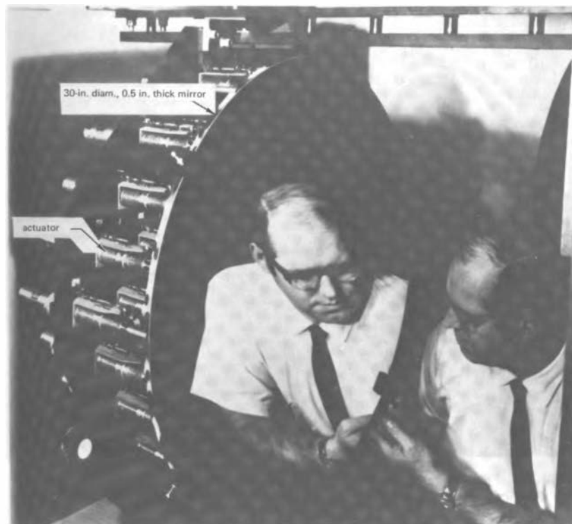
FIGURE 4 Flexible active-optics mirror.
