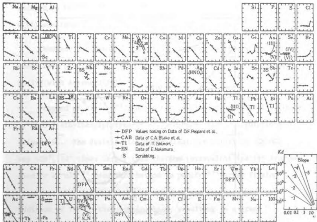
Figure 7. Extraction of Elements from HCl Solution by 50% HDEHP in Toluene as a Function of Acid Concentration. 178
