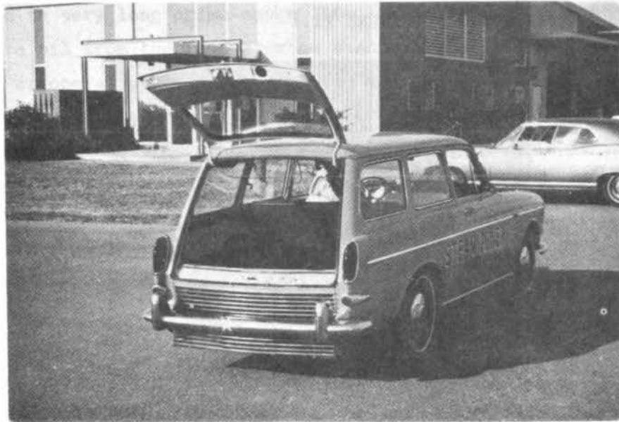
Rear View of VW with Carter Steam Engine Mounted. The Grill Covers the Boiler Stack and the Rear Condenser.
