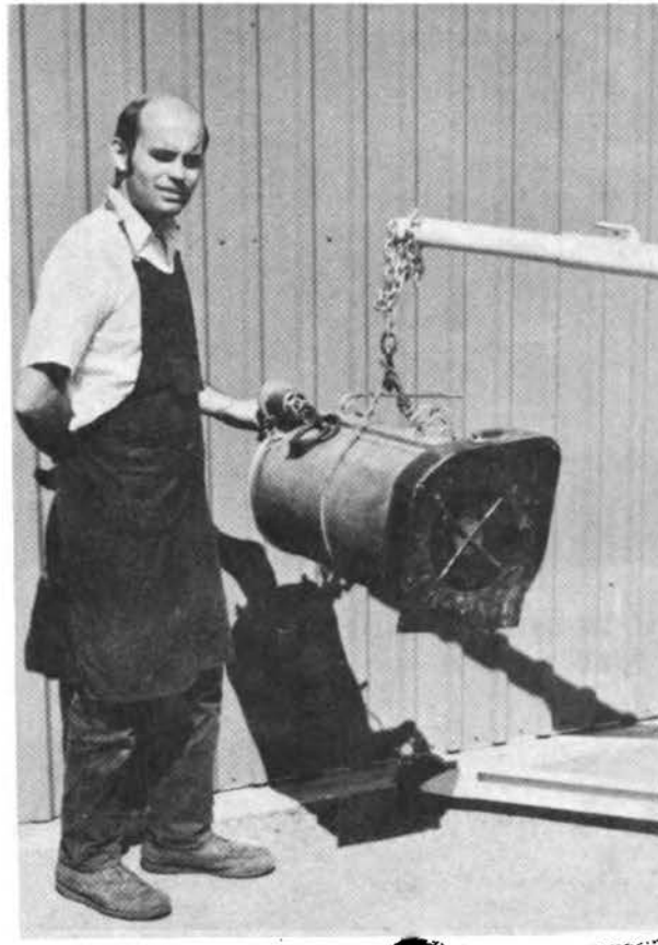
The Boiler-Burner Assembly.
