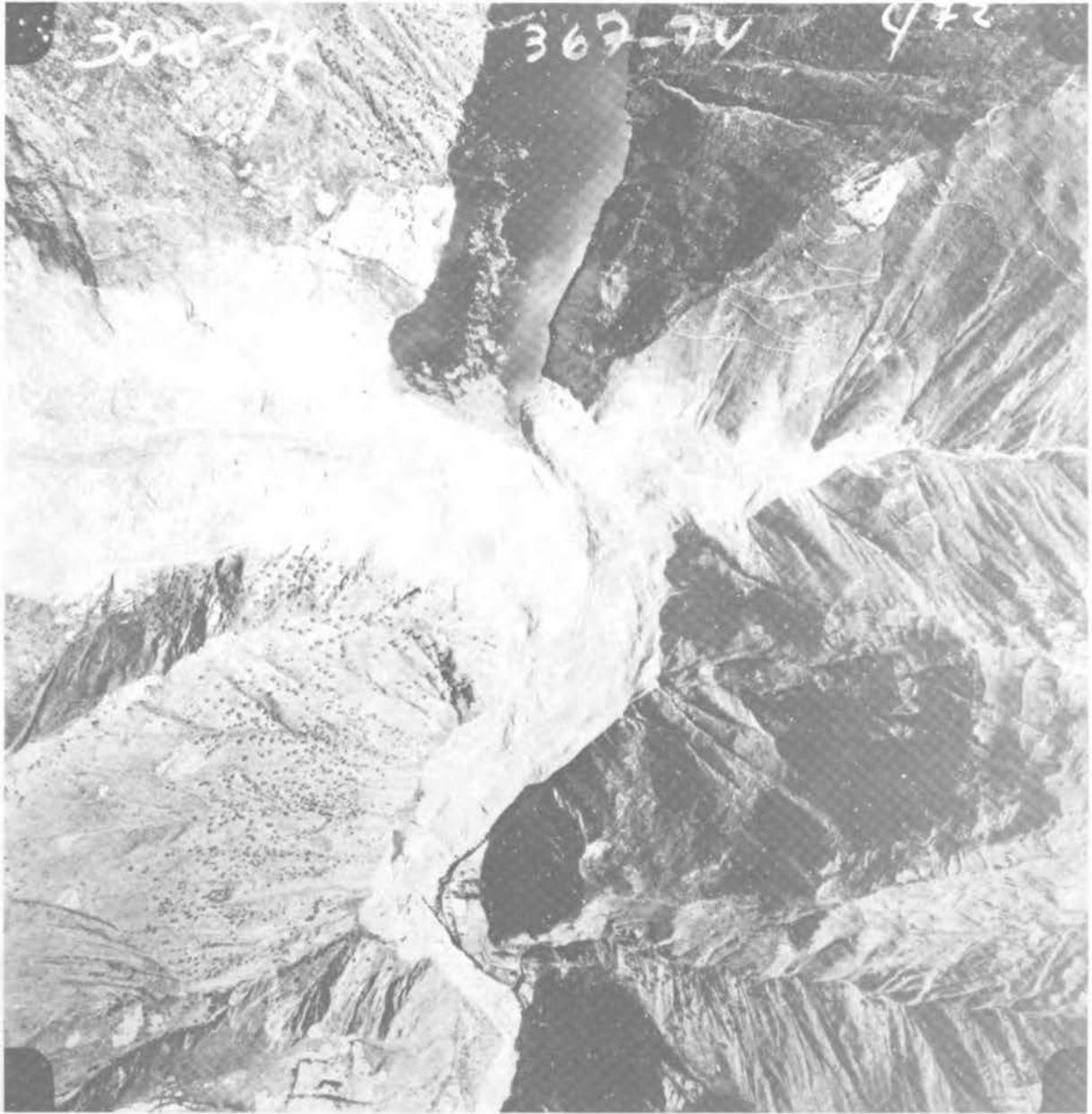
FIGURE 14. Vertical air photograph of the debris dam taken May 30, 1974 some nine days prior to the dam being overtopped. (Defensa Civil Photograph)
