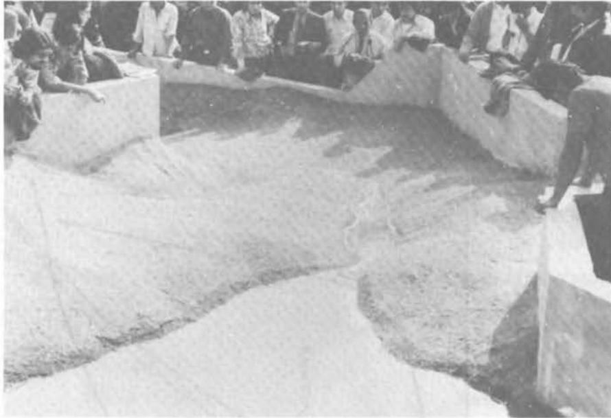
FIGURE 42. Hydraulic model, looking downstream at the stage where water just begins to trickle slowly over the debris dam.
