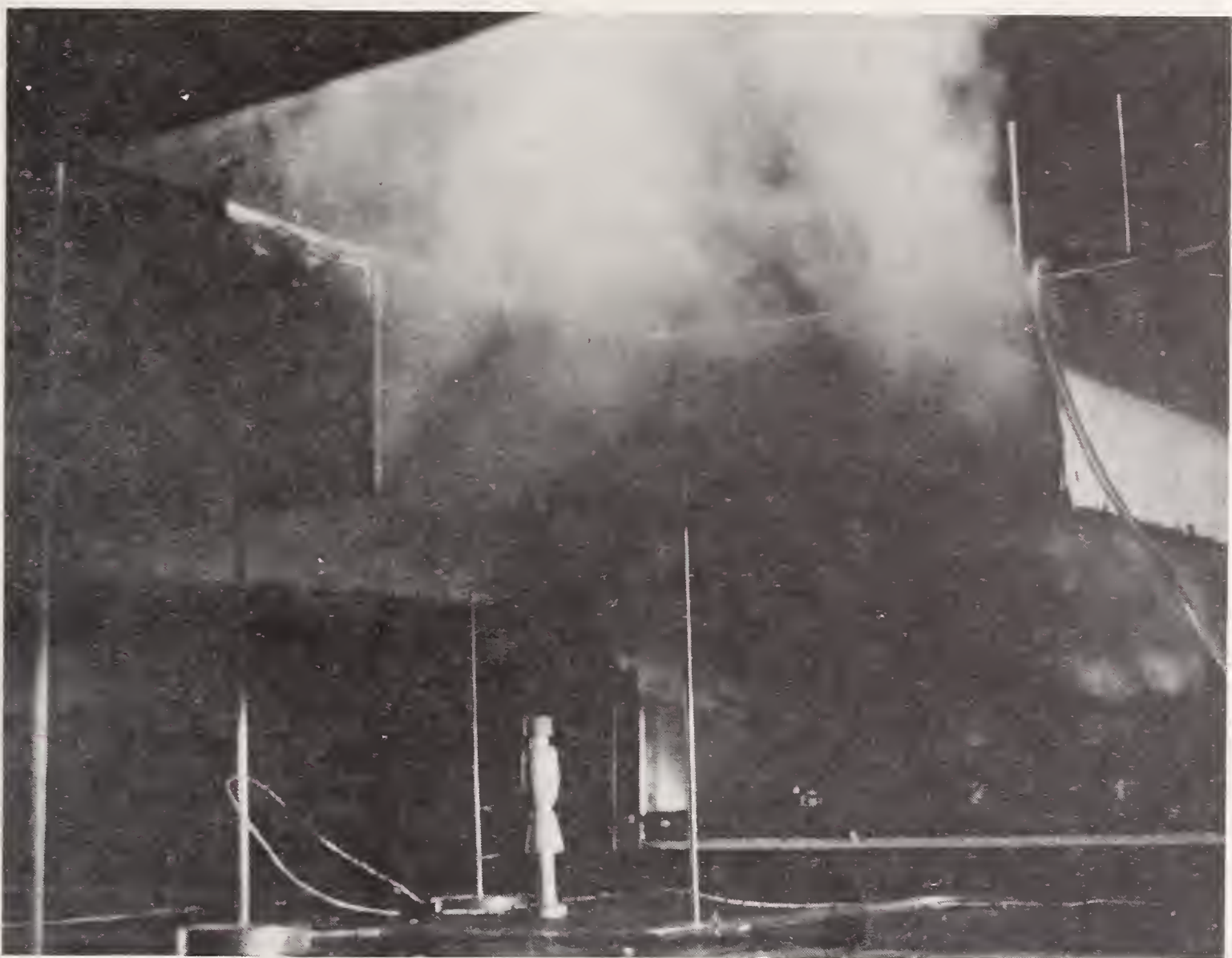
FIGURE 7 Smoke from a model fire confined by ceiling screens to form a compact plume.
