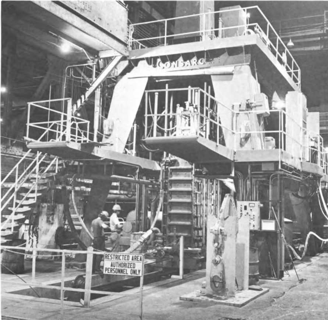
FIGURE 31 Lukens Steel ESR Slab Furnace of CONSARC Design (from Lukens Steel Company).
