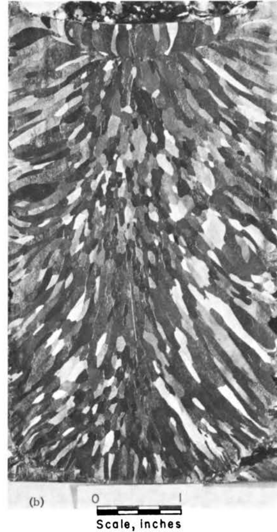
FIGURE 9 Comparative Macrostructures of ESR (a) and VAR (b) Molybdenum Ingots (from Calvert et al., 1971.)
