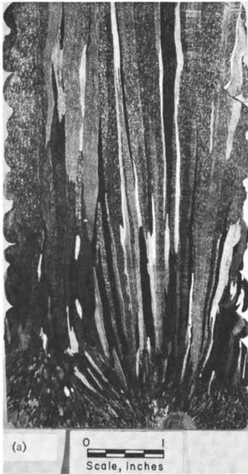
FIGURE 9 Comparative Macrostructures of ESR (a) and VAR (b) Molybdenum Ingots (from Calvert et al., 1971.)
