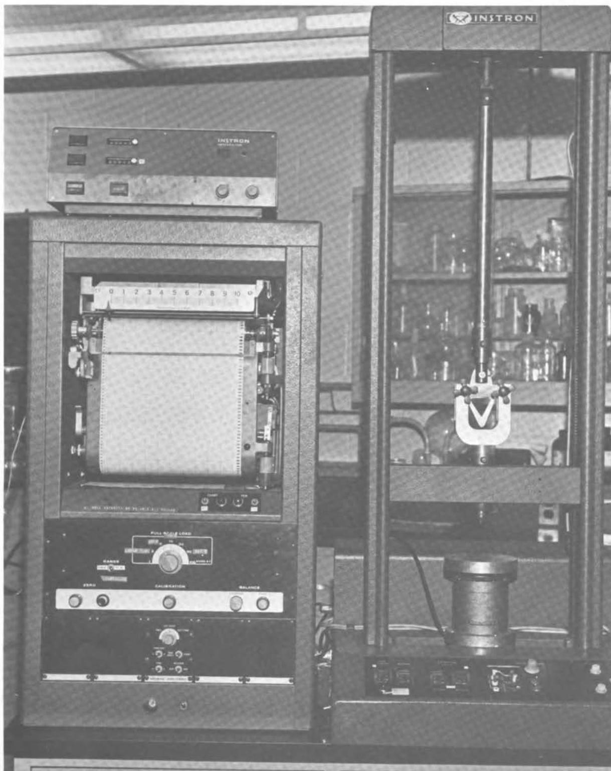
FIGURE 2 Instron Universal Testing Machine with Warner-Bratzler attachment.
