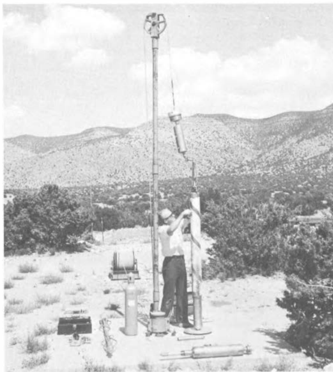
FIGURE 8 SRO borehole seismometer being prepared for installation. (Photo U.S. Geological Survey, Jon Peterson.)
