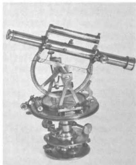
Below: Theodolite, a surveying instrument for measuring horizontal and vertical angles.
