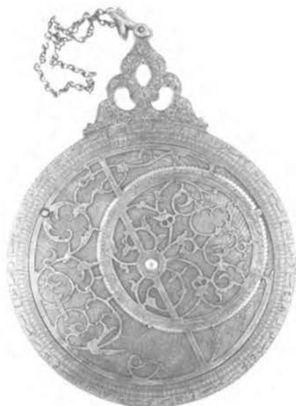
Above: Astrolabe, a surveying instrument for establishing astronomical position.
