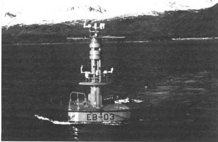
Large environmental (disk) buoy being prepared for anchoring in deep water off the coast of Alaska. (Courtesy, NOAA)
