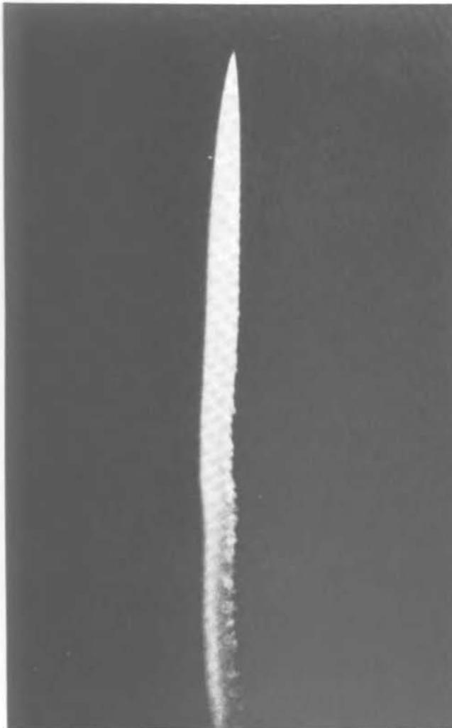
FIGURE 7.1 Portion of a trimethyl aluminum trail showing a release phase instability with vortex shedding on the right-hand edge 2 sec after release at 103 km.
