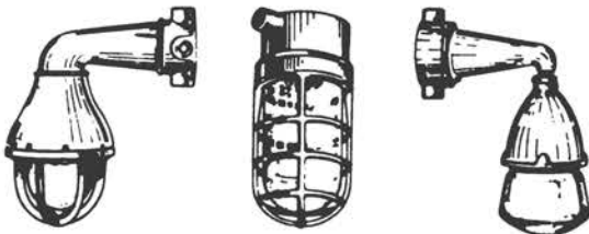
Fig. 2. Typical incandescent lighting fixtures for hazardous locations. Left, explosionproof. Center, enclosed gasketed. (See Table 1.) Right, dust-ignitionproof.
