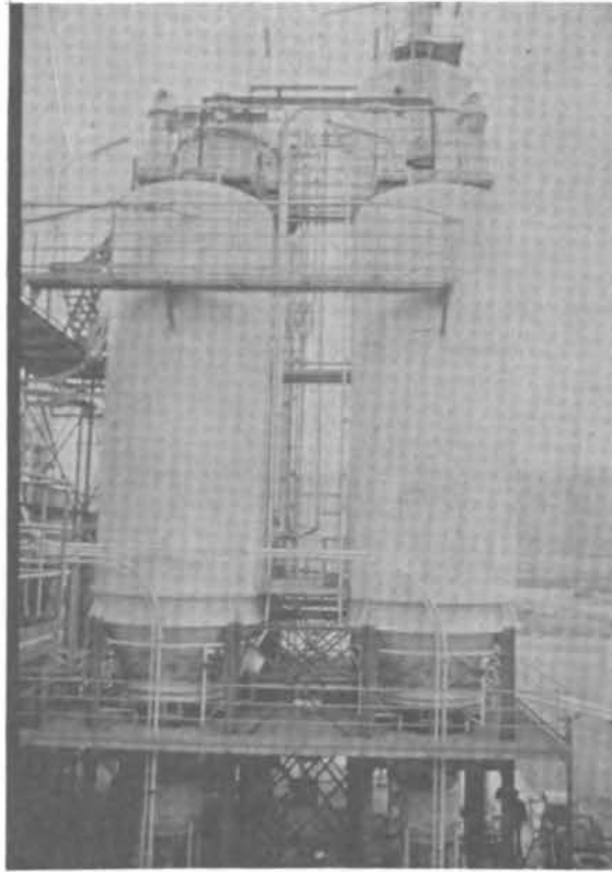
Fig. 35 : Vessel of a production plant; explosion pressure shock resistant design
