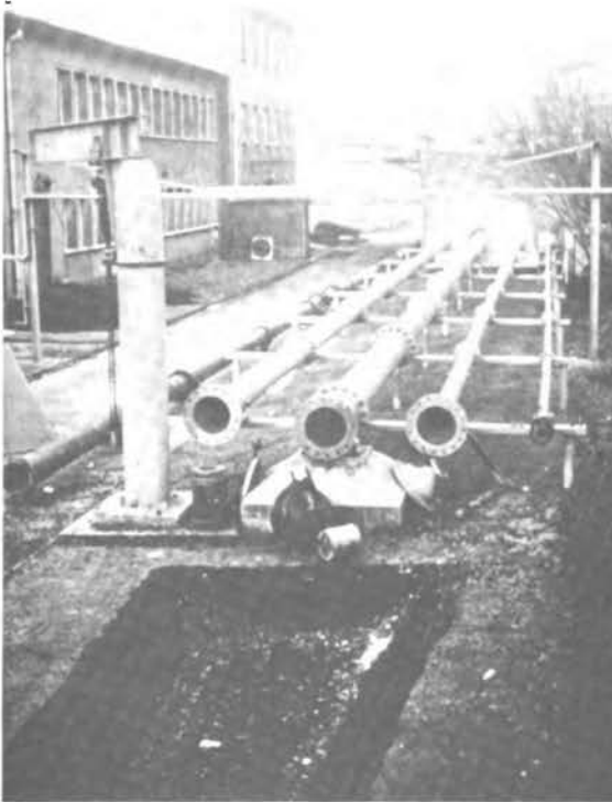
Fig. 23: Pipelines for basic research \varnothing 100 to 400 mm length 40 m
