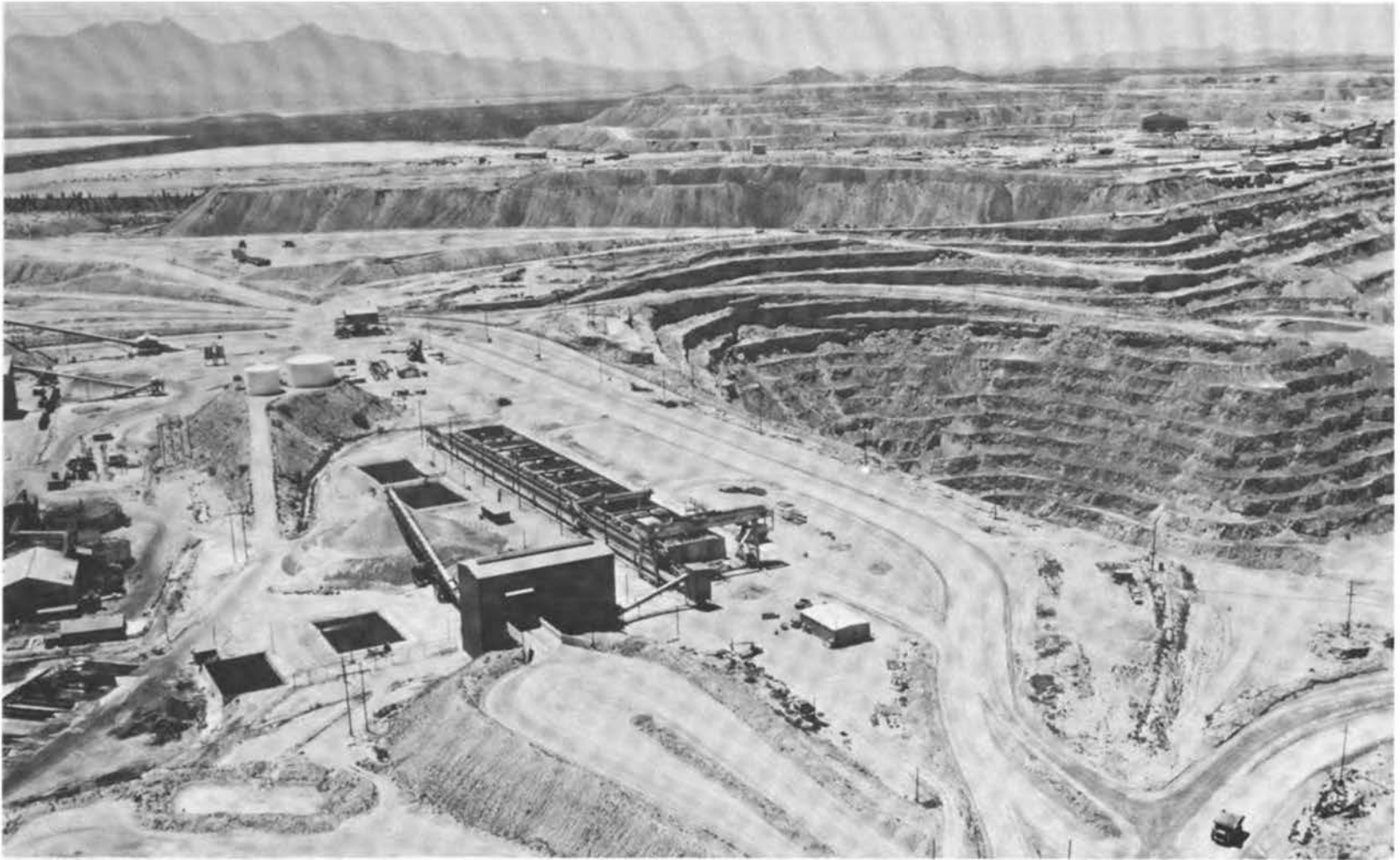
FIGURE 2.1 Part of the Sahuarita district south of Tucson, Arizona, where low-grade copper deposits are mined on a large scale by open-pit methods. Some processing facilities for one operation are adjacent to the pit in the foreground. Dumps of waste rock form the more distant terraced landscape. The nearly white areas in the left distance are surfaces of tailings ponds.
