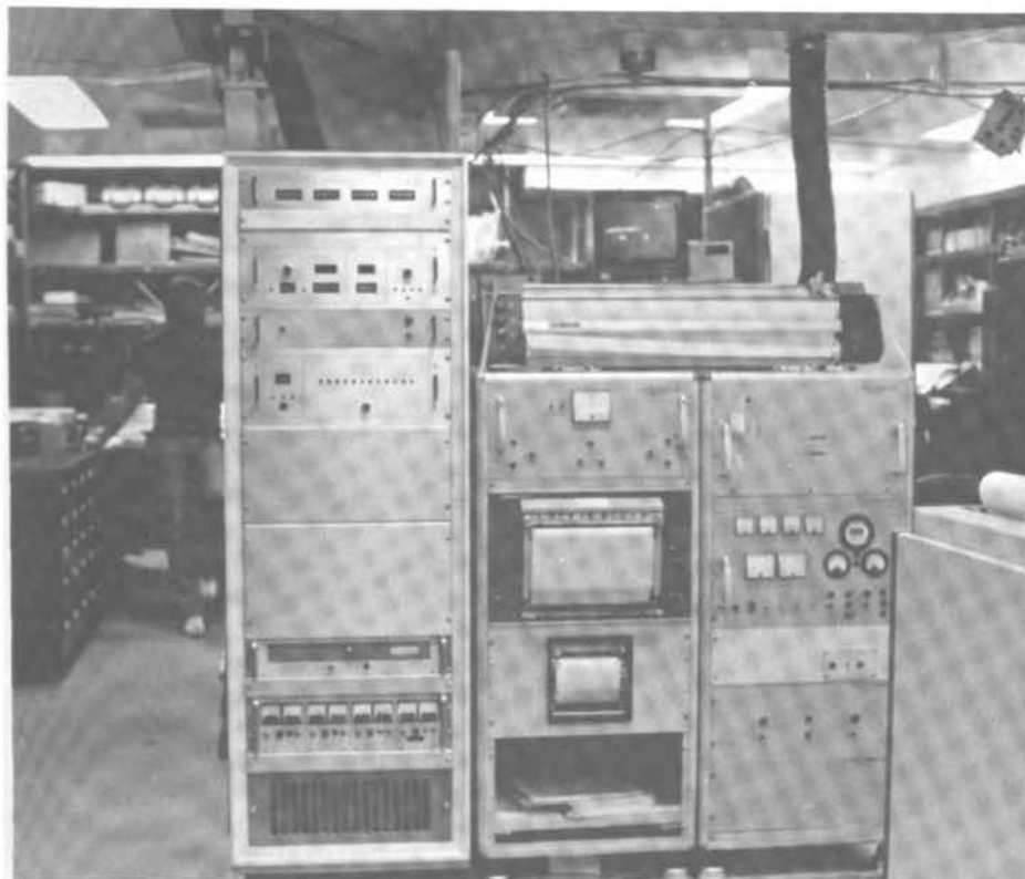
FIGURE C.14 Gravity-meter control electronics and WINS navigation system.
