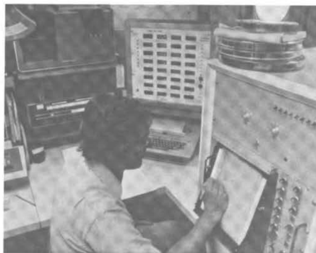
FIGURE C.11 Fiber optic camera (in foreground), EMR computer control unit, switch register, and CRT display.
