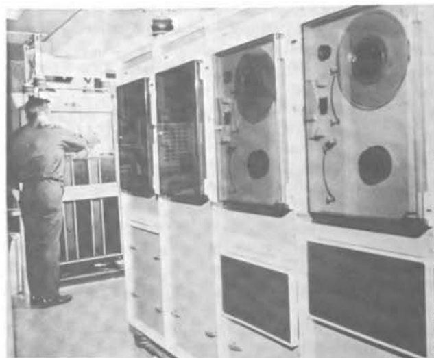
FIGURE C.18 Data logger and data processor magnetic tape units.
